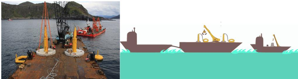
**Figure 3.** The WECs on the barge in Maren Test Site (left) and a schematic of the deployment (right): a towing boat dragging the barge with the two WECs and their buoys on top. The smaller boat is carrying the substation connected with the wires and the cable drum. Both boats have cranes.
