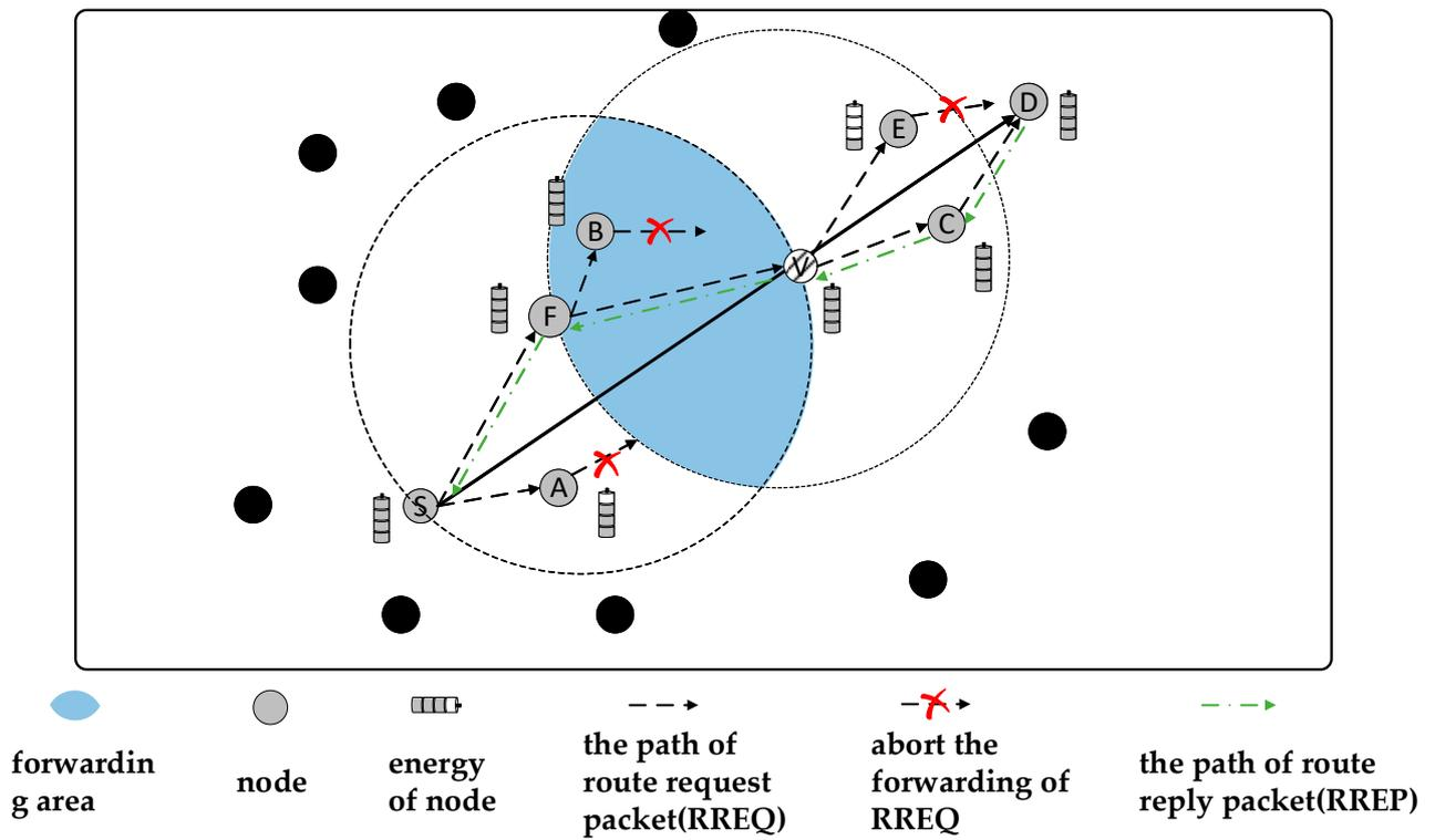
Figure 3. Forwarding area of RFAODV (last forwarding node is F, S-F-V-C-D is the ideal route).
