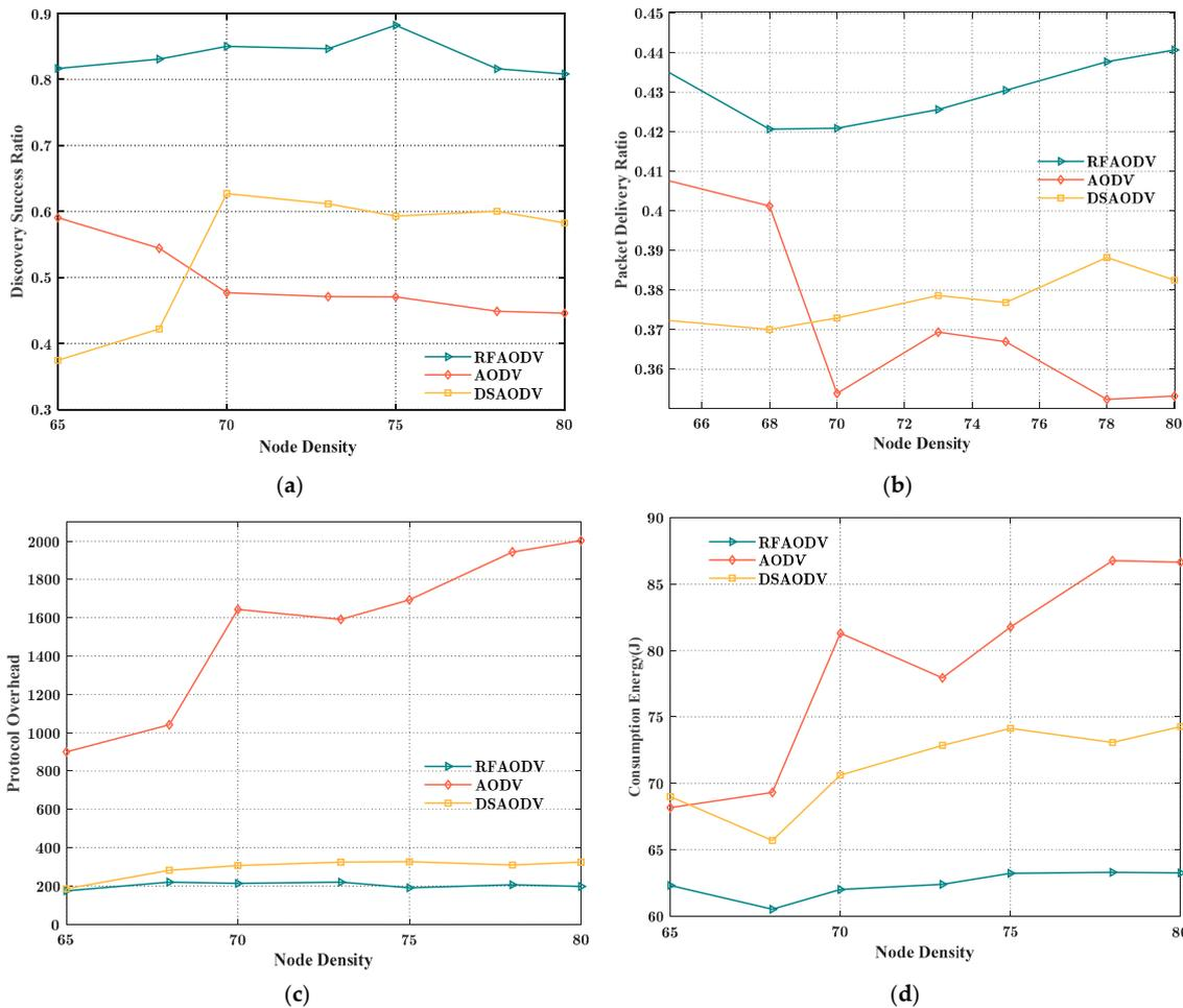
**Figure 7.** Effects of the node density. (a) Discovery success ratio vs node density; (b) packet delivery ratio vs node density; (c) protocol overhead vs node density; (d) consumption energy vs node density.
