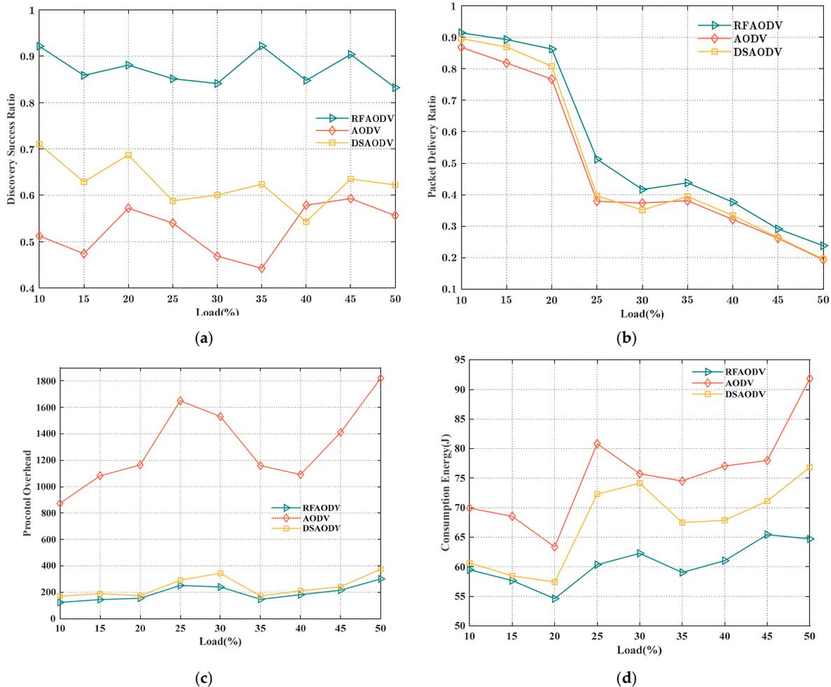
**Figure 6.** Effects of the traffic load. (a) Discovery success ratio vs load; (b) packet delivery ratio vs load; (c) protocol overhead vs load; (d) consumption energy vs load.
