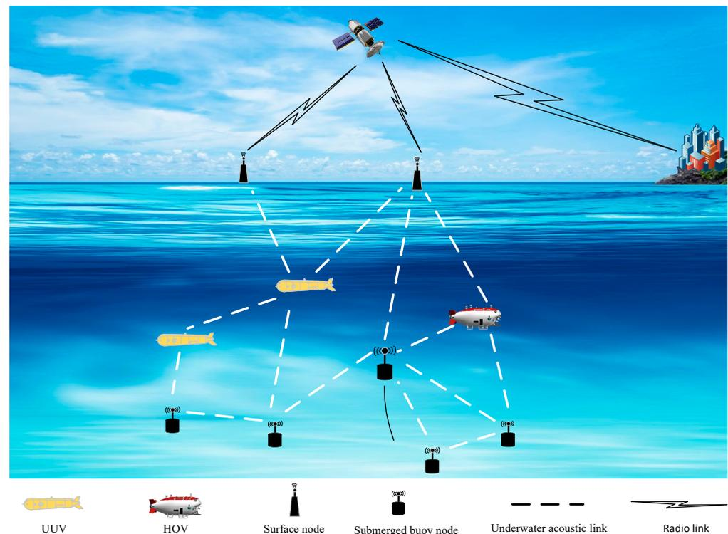
**Figure 1.** Architecture of underwater wireless sensor networks.
