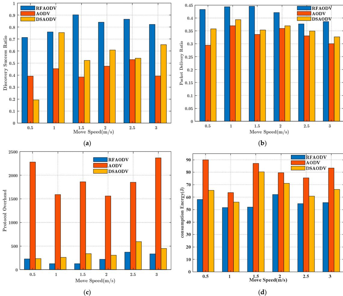
**Figure 8.** Effects of the move speed. (a) Discovery success ratio vs move speed; (b) packet delivery ratio vs move speed; (c) protocol overhead vs move speed; (d) consumption energy vs move speed.
