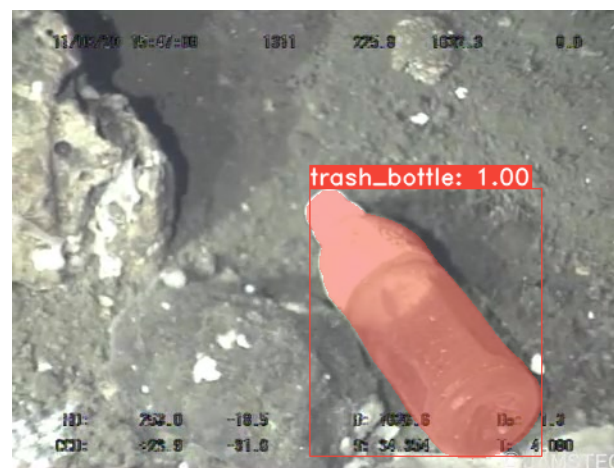
Figure 1. Instance segmentation example using YOLACT with the IoU metric.
