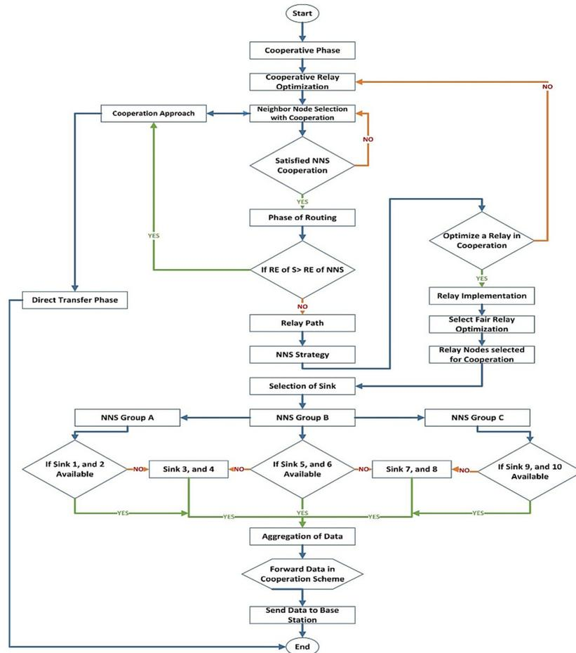
Figure 3. Functionality flowchart of the proposed CR-NBEER protocol.
