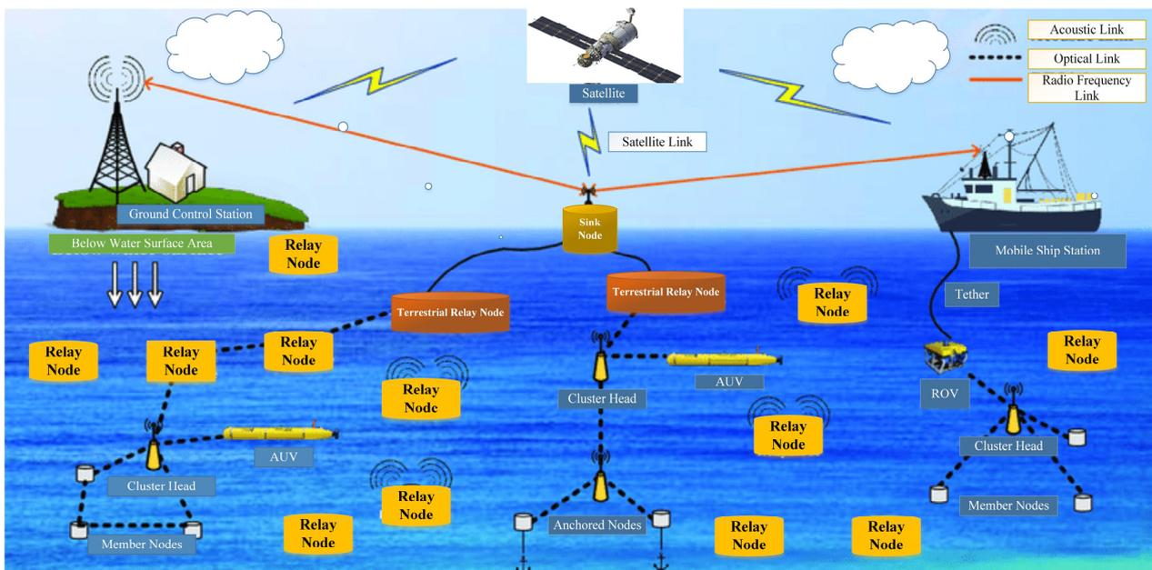
Figure 1. Illustration of cooperative relay-based scheme for MUSN.
