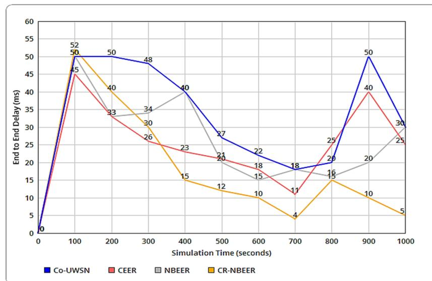
**Figure 4.** EED of existing and proposed methods vs. simulation time.
