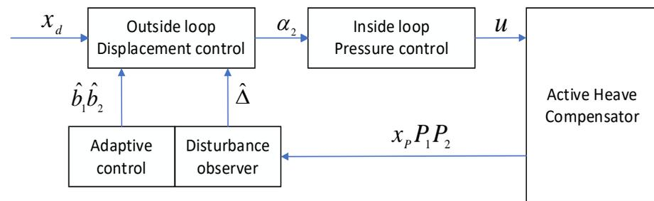
Figure 7. Block diagram of DOB-ANCC controller structure.
