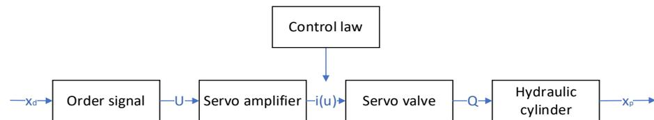
Figure 5. Working schematic diagram of crane AHC electro-hydraulic servo system.
