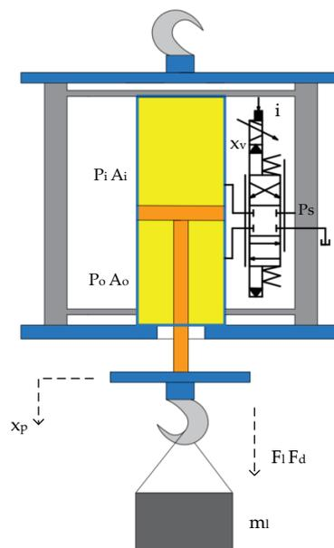
Figure 4. Schematic diagram of the AHC system.
