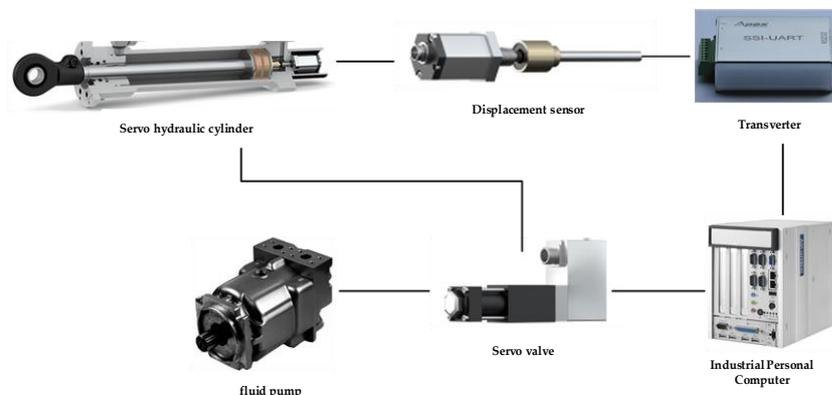
Figure 6. Actual control elements of active heave compensation system.
