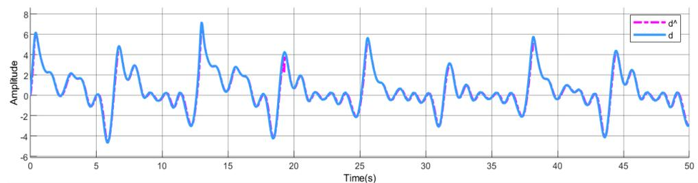
Figure 8. Tracking performance of disturbance observer.
