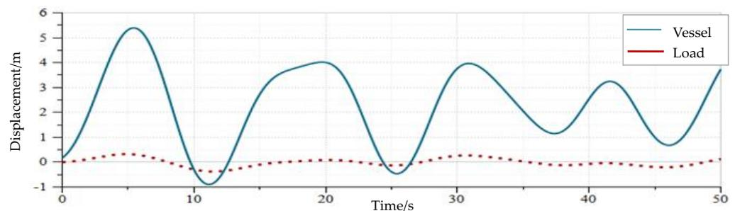
Figure 14. Displacement curves of vessel and load under a random wave.
