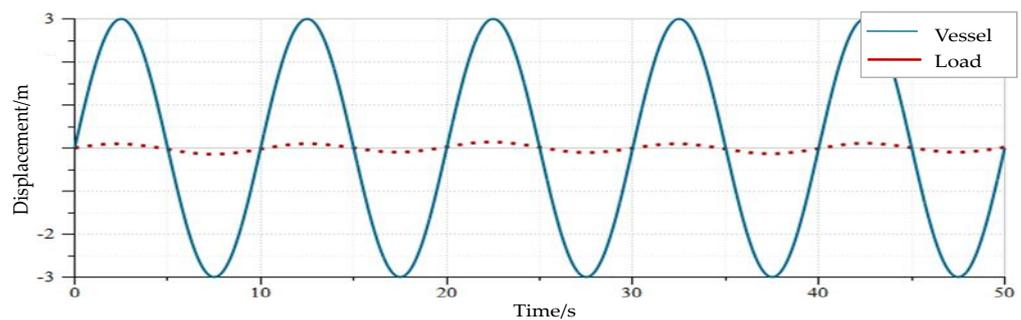
Figure 13. Displacement curves of vessel and load under four sea conditions.
