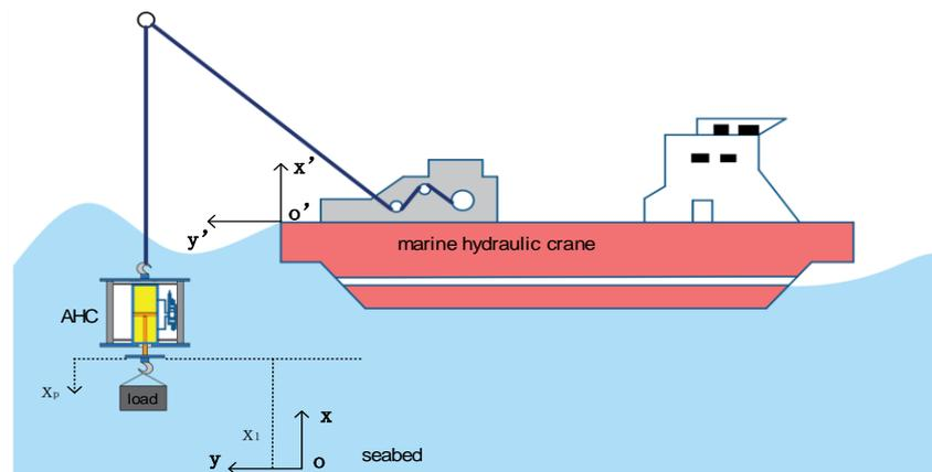
Figure 3. Layout of AHC system on marine crane.
