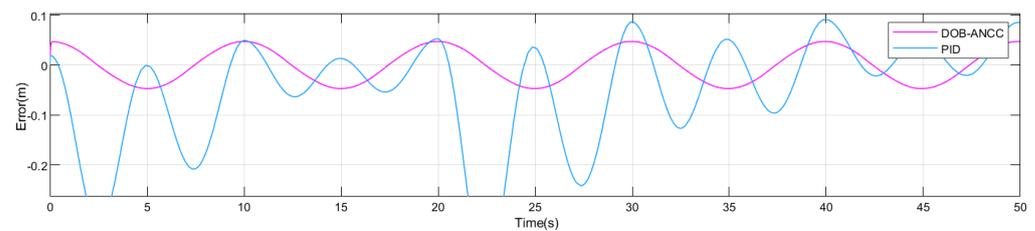
Figure 11. Tracking error of different controllers.
