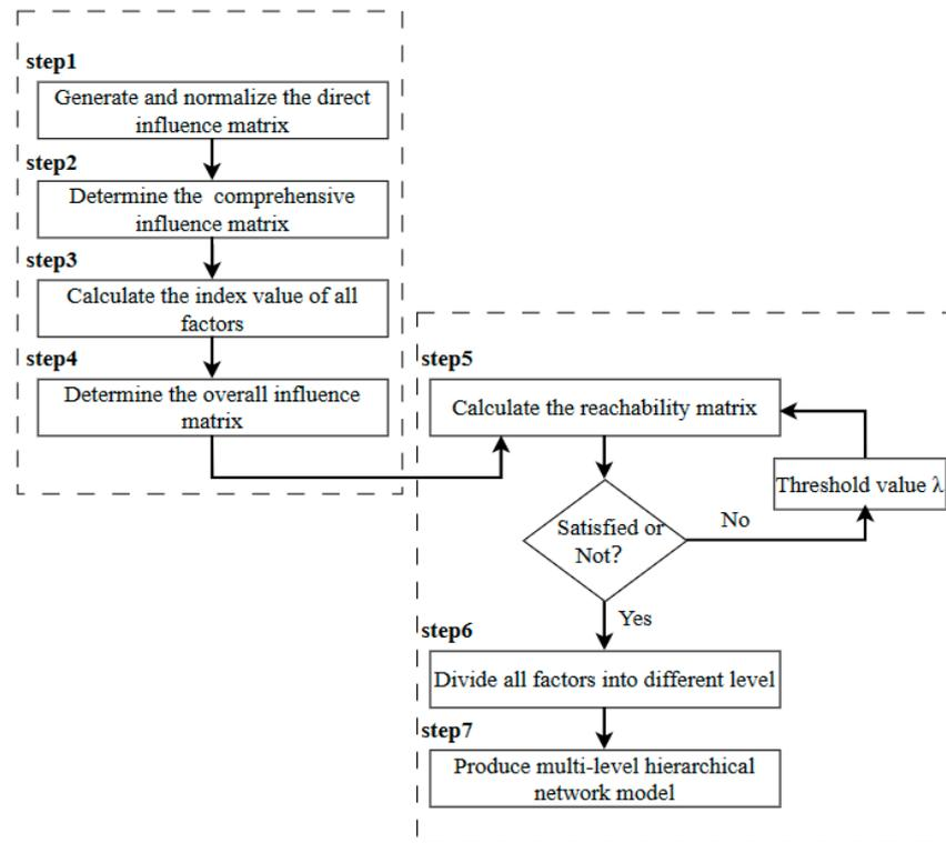
Figure 2. The production of the DEMATEL-ISM model.
