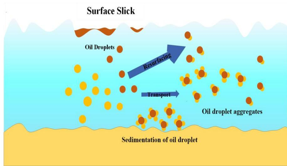
Figure 6. Conceptual model of oil particle aggregate.
