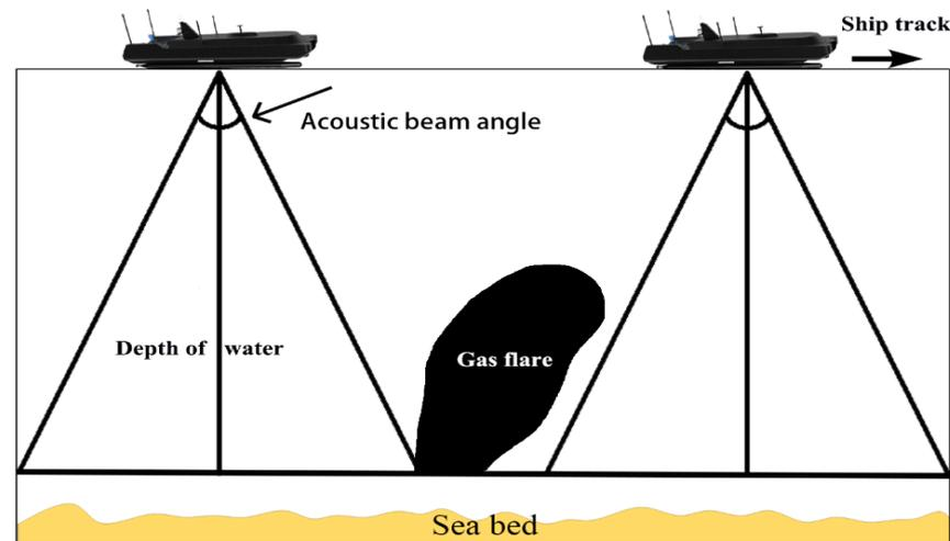
**Figure 5.** Acoustic bubble monitoring.
