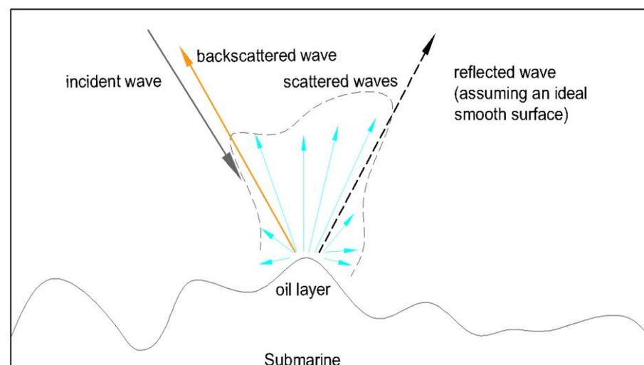
**Figure 3.** The principle of the acoustic wave (back) scattering phenomenon. (The black solid line represents the incident wave. the yellow solid line represents the backscattered wave. The black dashed line represents the reflected wave. The blue line in the dashed box represents the scattered wave. The blank part represents the seawater medium, and the black curve below represents the oil layer medium.).
