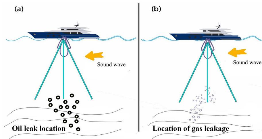
**Figure 4.** (a) Acoustic monitoring of oil droplets; (b) acoustic monitoring of leaking gas.
