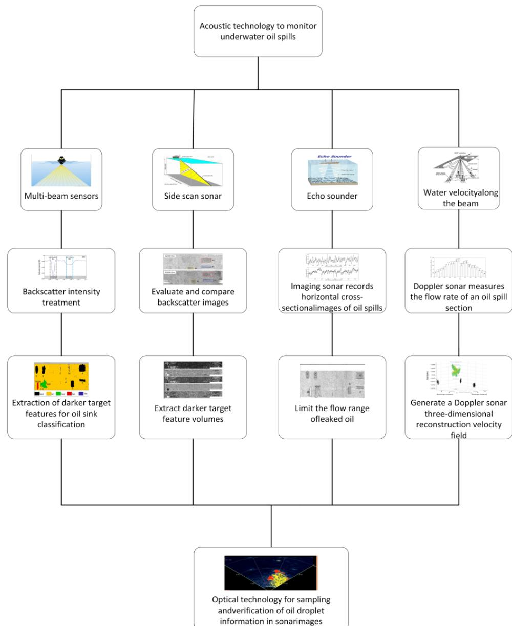
Figure 8. Four kinds of acoustic instruments oil spill monitoring process.
