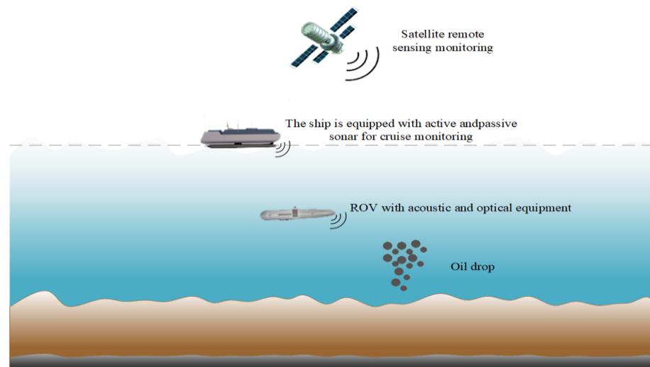
**Figure 9.** Shipboard acoustic monitoring and underwater robotic monitoring of oil spills.
