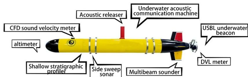
**Figure 10.** Underwater robots equipped with multiple acoustic detectors.
