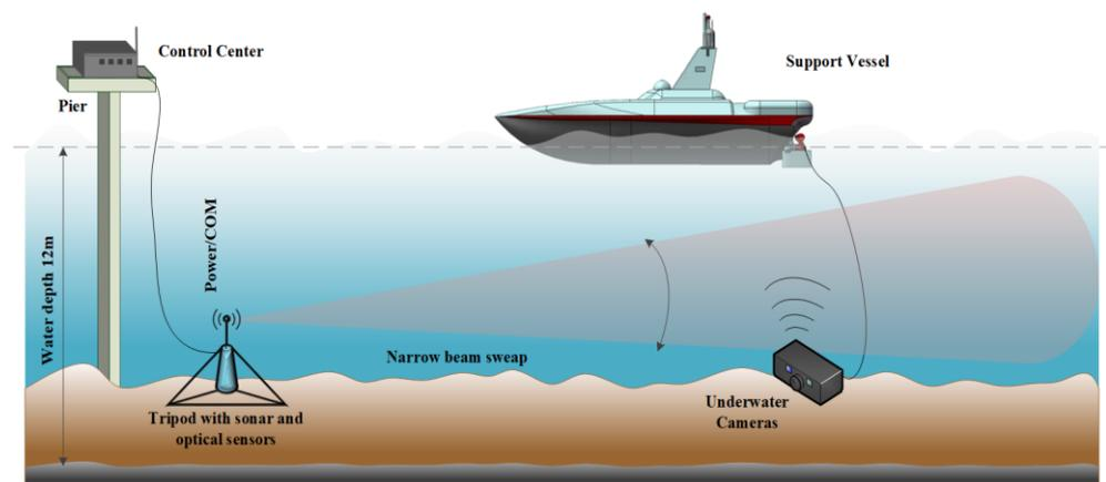
**Figure 7.** Acousto-optic technology monitoring.
