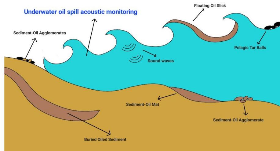
**Figure 2.** Conceptual model of various oil residues found in nearshore environments.
