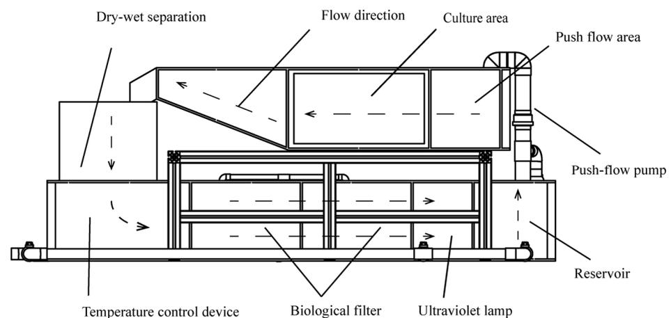
**Figure 1.** Circulating water culture tank.
