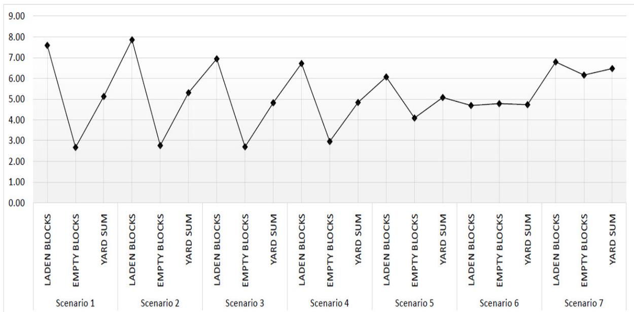
**Figure 7.** YC waiting time (min). It represents the average waiting time of all YCs, as well as separately the average waiting times of YCs positioned in the full container zone and the average waiting time of YCs in the empty container zone.
