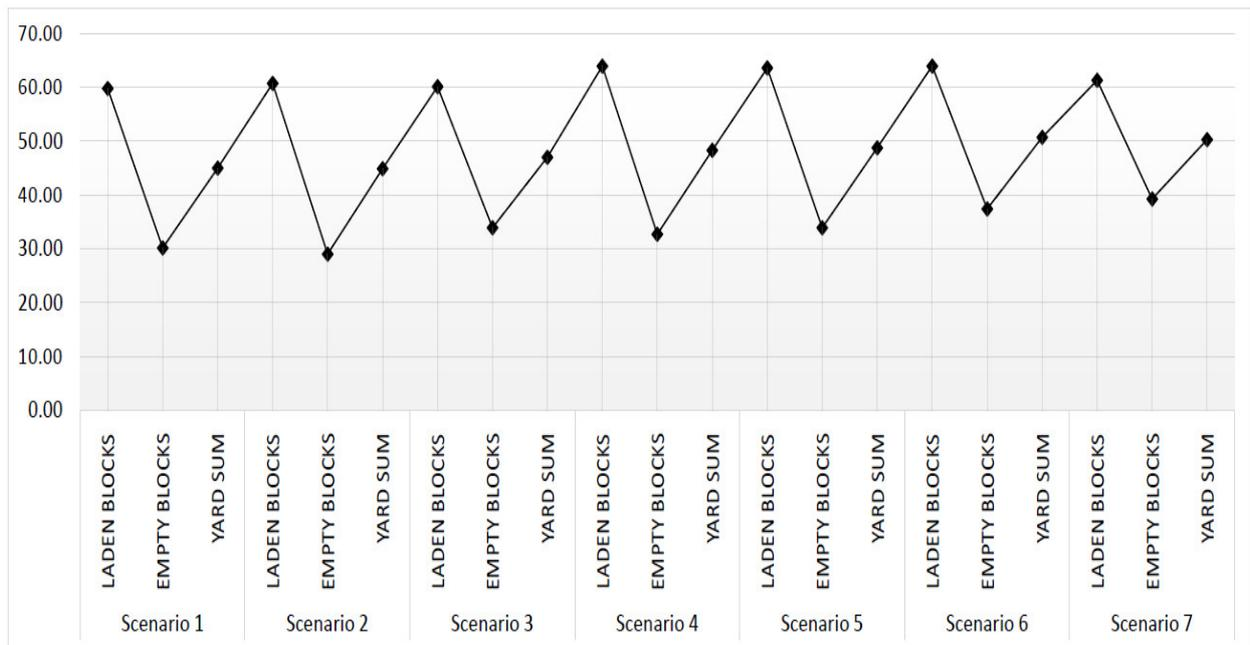
**Figure 6.** Yard utilisation (%). The average occupancy of the whole yard area as well as separately, i.e., the average occupancy of a zone with blocks for full containers as well as a zone with blocks for empty containers for all seven simulated scenarios.
