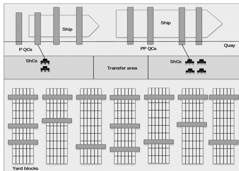
Figure 1. Perpendicular terminal layout.
