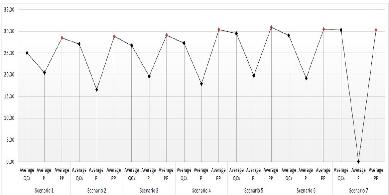
**Figure 5.** QC moves per hour. The average number of moves per hour performed by the P QCs and the PP QCs. It also shows the average total number of moves per hour by all eight QCs in seven simulated scenarios.
