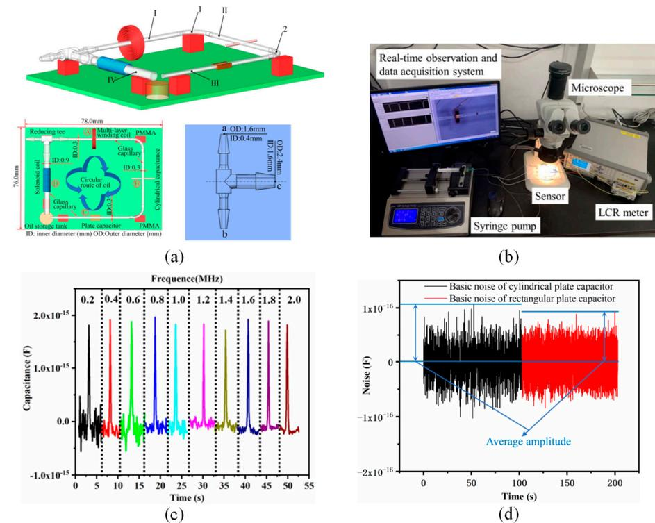
**Figure 5.** High-sensitivity, high-throughput capacitive detection sensor for oil contamination [76]. (a) The overall structure design of the sensor. (b) Capacitive sensor experimental test system. (c) The detection signals obtained by the cylindrical capacitive sensor under different excitation frequencies. (d) Basic noise of different types of capacitive sensors.
