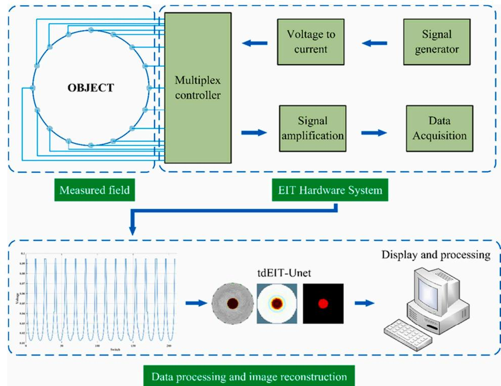
Figure 7. Image processing sensor for oil wear particles based on tdEIT and Unet [85].
