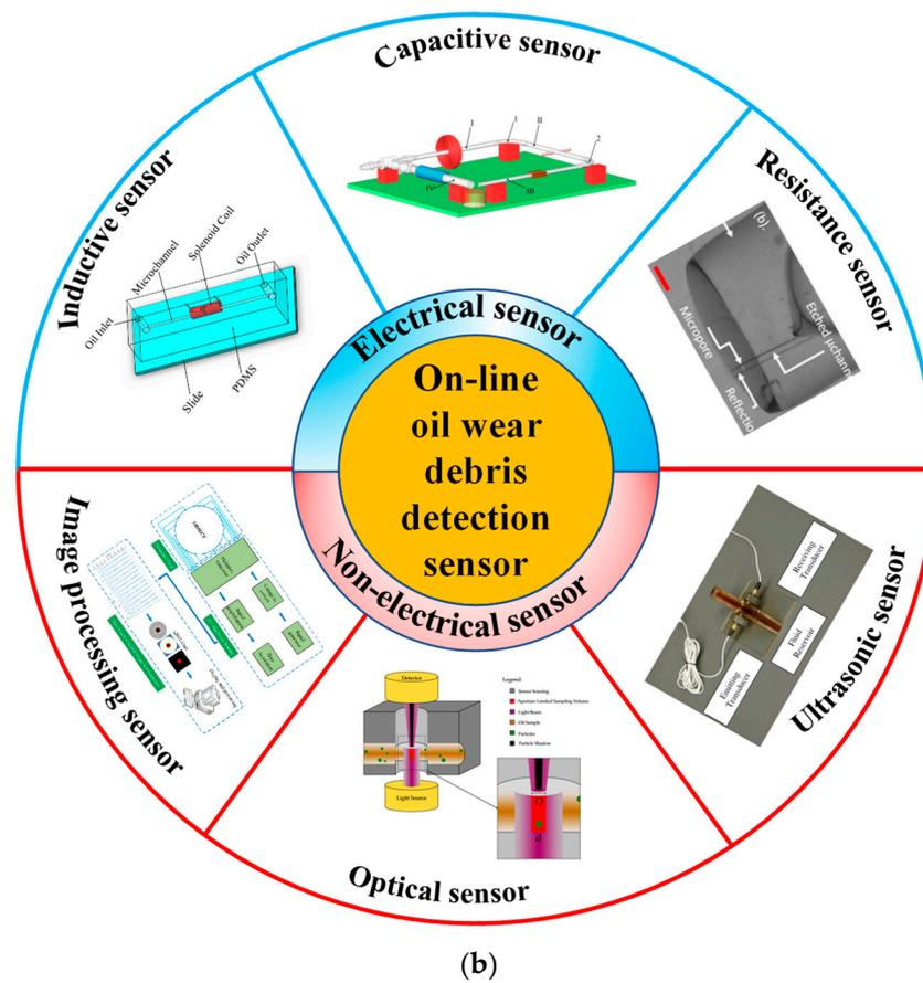
**Figure 1.** (a) Oil particle analysis monitoring location [16] (b) Classification diagram corresponding to the on-line oil wear debris detection sensor employed for monitoring the wear state of marine equipment [43,72,79,85,92,100].
