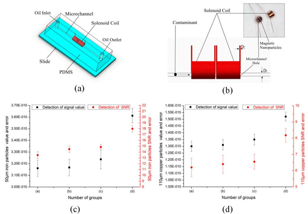
**Figure 2.** Inductive wear particle detection sensor based on PDMS [43]. (a) Structural design of inductive sensor. (b) Schematic diagram of wear particles passing through the sensor. (c) The detection results of iron particles with a diameter of 50  $\mu\text{m}$  in the inductive detection sensor. (d) The detection results of copper particles with a diameter of 100  $\mu\text{m}$  in the inductance detection sensor.
