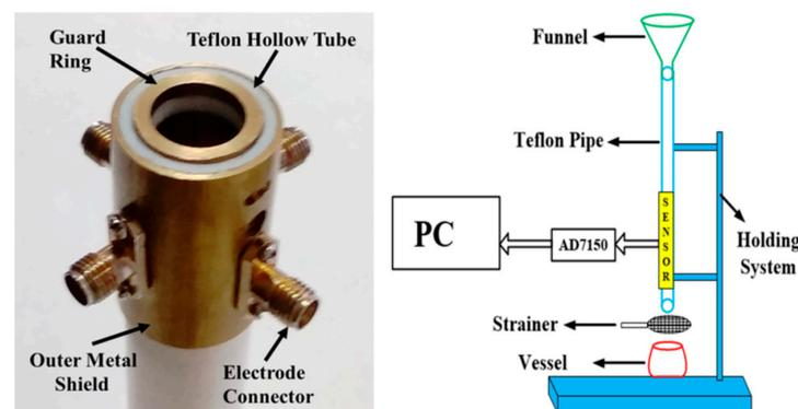
**Figure 4.** High-precision cross-capacitive metal particle detection sensor [72].
