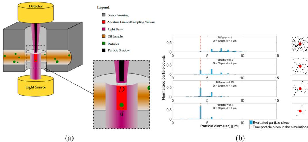
**Figure 8.** Optical sensor for evaluating wear particle distribution in lubricating oil systems [92]. (a) Detection principle of optical sensor. (b) A random sample of pore size and particle position was evaluated using an optical sensor for different concentrations of 4 μm particles.
