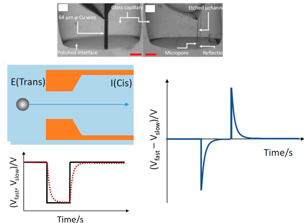
Figure 6. Detection principle of resistive particle detection sensor [79].
