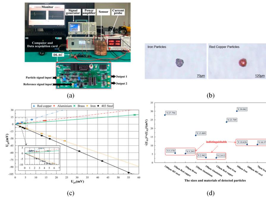
**Figure 3.** Inductive wear particle detection sensor based on dual lock-in amplifier circuit [57]. (a) Experimental system components for particle detection. (b) Microscopic images of iron particles with a diameter of 70 µm and copper particles with a diameter of 120 µm. (c) Complex plane distribution plot of particles of different sizes and materials. (d) The detection results obtained by real domain detection.
