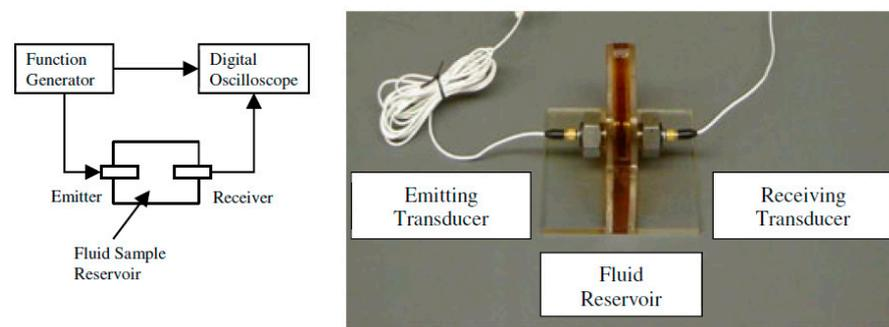
**Figure 9.** Ultrasonic sensors for oil viscosity and wear particle detection [100].
