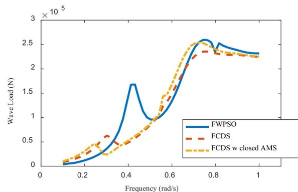
Figure 7. Second-order wave load transfer functions of surge.
