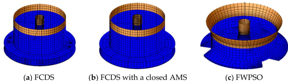
**Figure 4.** Panel models of the FCDS and FWPSO.
