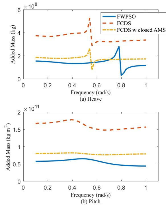
Figure 5. Added mass of the heave and pitch.
