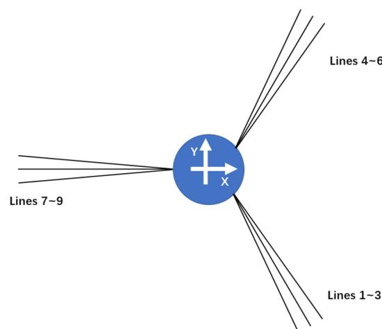
**Figure 9.** Configuration of the mooring system.
