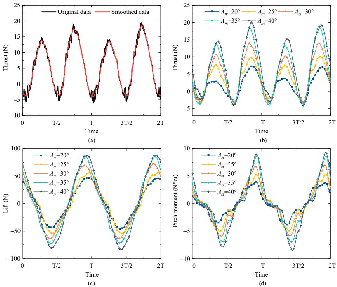
**Figure 9.** Data smoothing and comparison. (a) Comparison of the original data and smoothed data. (b) Thrust variation with time ( $f = 0.34$  Hz,  $\Delta\varphi = 10^\circ$ ). (c) Lift variation with time ( $f = 0.34$  Hz,  $\Delta\varphi = 10^\circ$ ). (d) Pitching moment variation with time ( $f = 0.34$  Hz,  $\Delta\varphi = 10^\circ$ ).
