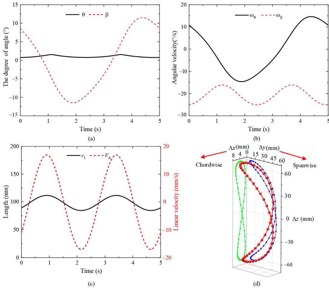
**Figure 4.** Motion analysis results of the bionic pectoral fin. (a) The curves of  $\theta$  and  $\beta$  changes over time. (b) The curves of  $\omega_\theta$  and  $\omega_\beta$  changes over time. (c) The curves of  $r_1$  and  $V_A$  changes over time. (d) The spatial trajectories of the left pectoral fin coordinate origin  $o_1$ .
