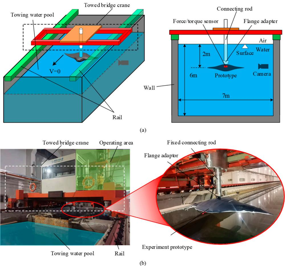
**Figure 6.** The composition of the experimental system. (a) The composition of the towing water pool and the installation diagram of the experimental prototype. (b) The actual experiment scene.
