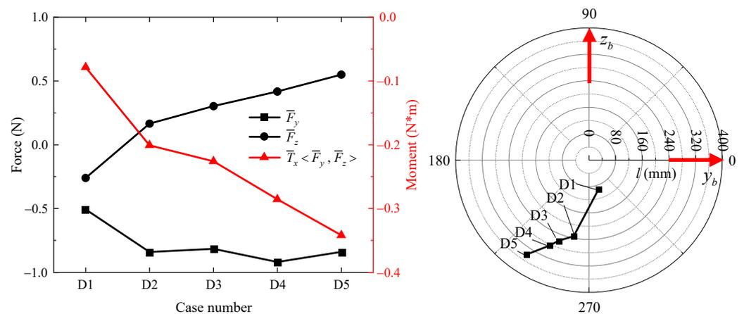
Figure 13. Hydrodynamic performance and equivalent point variation in Case D.
