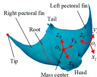
**Figure 1.** Coordinate frames of the rays.
