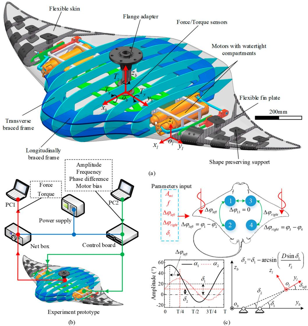
**Figure 5.** Composition and configuration of the experimental system. (a) Mechanical composition of the experimental prototype. (b) Cable connection and data flow of the experimental prototype. (c) Diagram of the CPG control strategy Adapted from the Ph.D. dissertation of Cao Yong (2015, Beihang University) [28] and definition of the pectoral fin bias.
