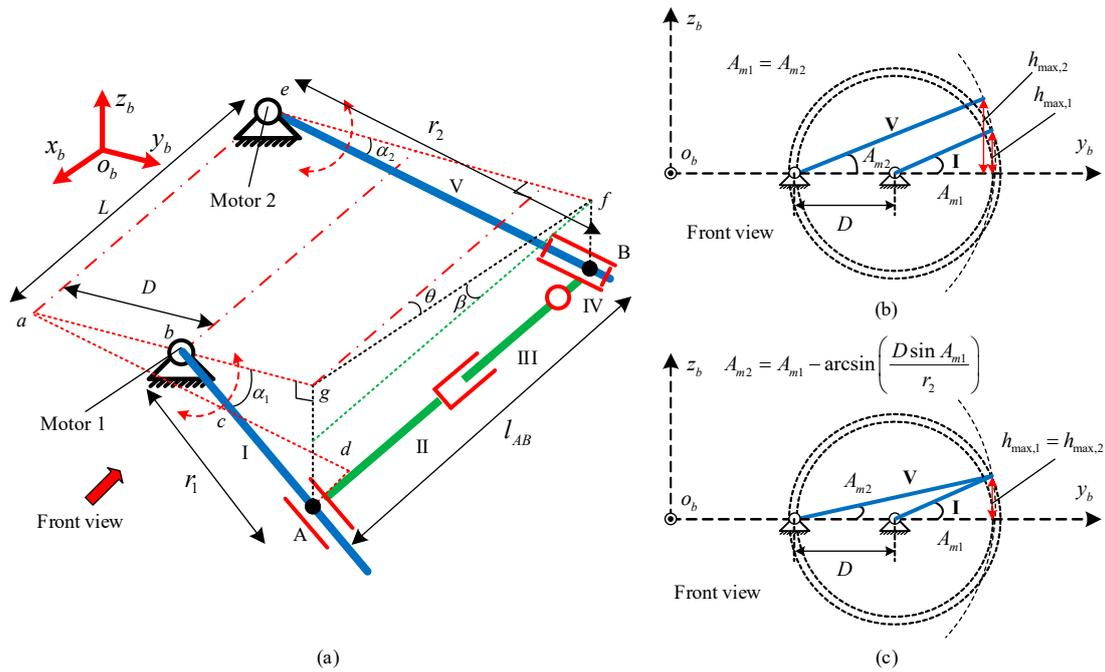
**Figure 3.** Geometric relationship of the bionic pectoral fin mechanism. (a) Schematic diagram of bionic pectoral fins. (b) Geometric relationship between the driving components without compensation. (c) Geometric relationship between the driving components after compensation.
