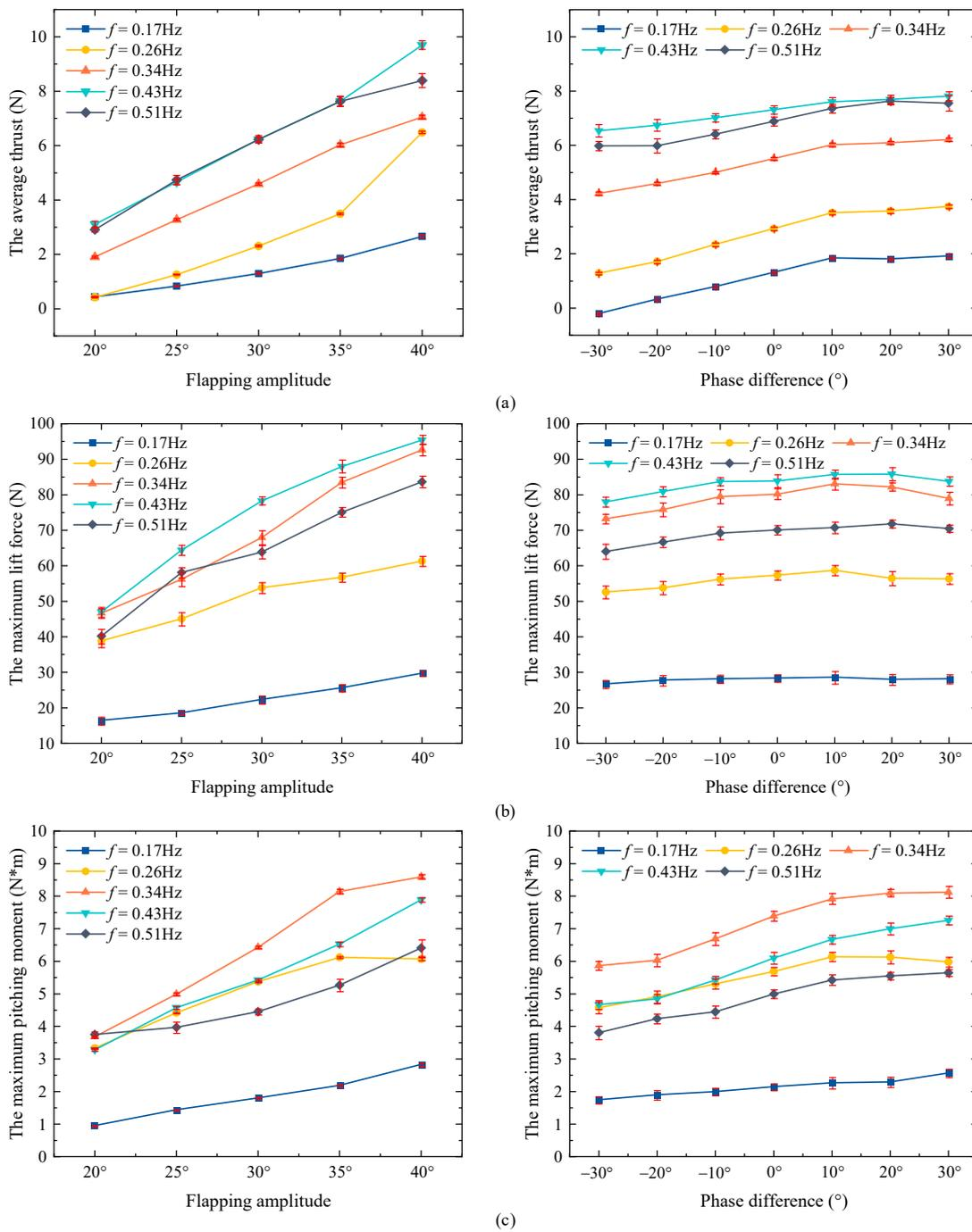
**Figure 10.** Influences of different oscillation parameters on the hydrodynamic performance. (a) The influence on average thrust. (b) The influence on the maximum lift. (c) The influence on the maximum pitching moment.
