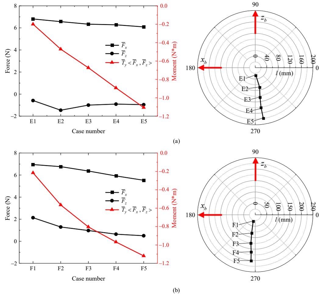
**Figure 14.** Hydrodynamic performance and equivalent point variation in pitching torque. (a) Experimental results of Case E. (b) Experimental results of Case F.
