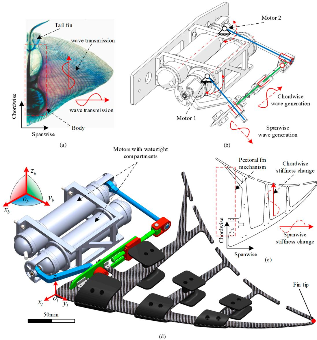
**Figure 2.** Mechanical design of the pectoral fin. (a) Calcification of the pectoral fin skeleton, adapted from the research article of Justin T. Schaefer (2005, Wiley) [15]. Red areas indicate calcification, and blue areas indicate cartilage. (b) Spatial linkage mechanism. (c) Fin plate with uniform thickness. (d) The 2-DOF bionic pectoral fin.
