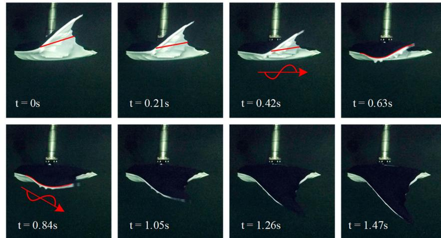
**Figure 8.** Morphological changes in the pectoral fin during the downstroke ( $A_m = 35^\circ$ ,  $f = 0.34$  Hz, and  $\Delta\varphi = 30^\circ$ ).
