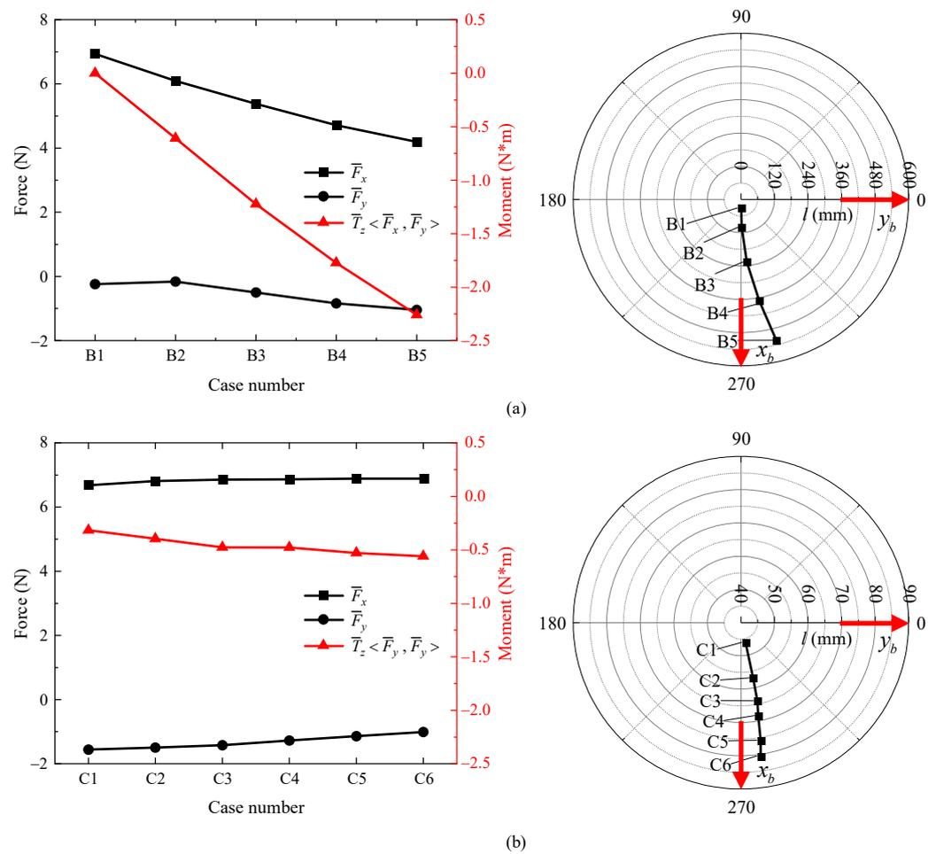
Figure 12. Hydrodynamic performance and equivalent point variation in turning torque. (a) Experimental results of Case B. (b) Experiment results of Case C.
