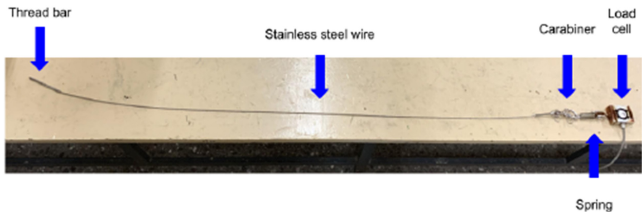
Figure 3. The mooring line used in the experiment.
