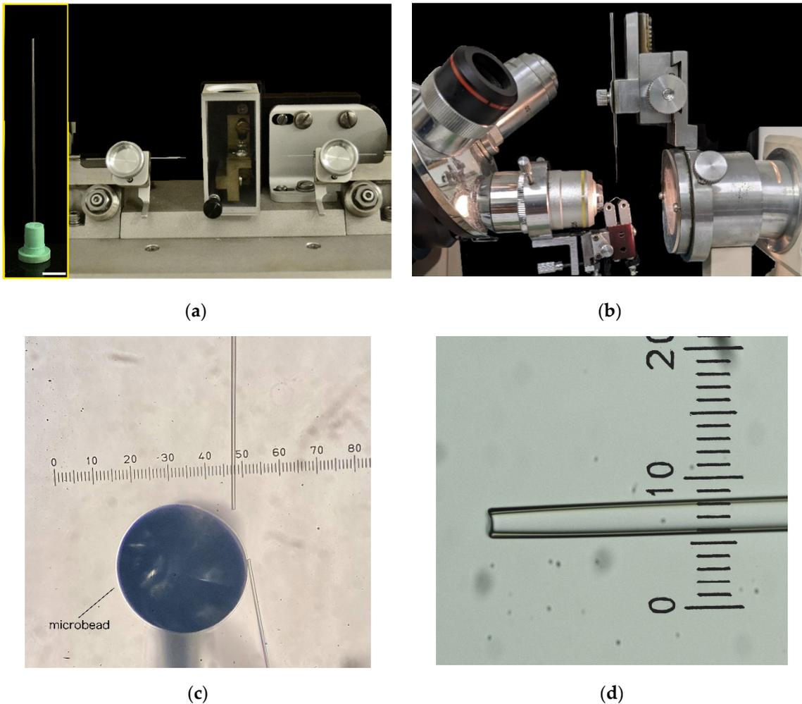
**Figure 1.** Preparation of the capillary before the picking procedure: (a) Borosilicate capillary before the cut and Flaming/Brown micropipette puller holding the cut capillary; (b) Cutting and bending of the capillary through a microforge; (c) Cut capillary of 10  $\mu\text{m}$  inner diameter; (d) Cut capillary of 20  $\mu\text{m}$  inner diameter. Scale bars are also reported.
