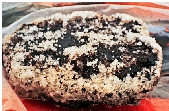
Figure 3. A piece of ice recovered from an area that had undergone a spill (Photograph from Environment Canada). The oil is in small particles throughout this piece of ice.
