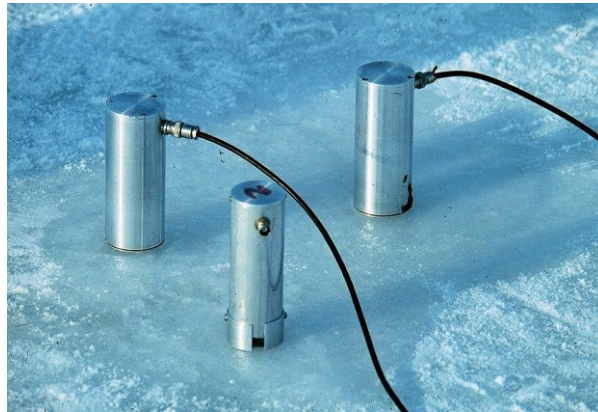
Figure 2. Transducers placed on sea ice for a field test of acoustic measure to detect oil under ice.
