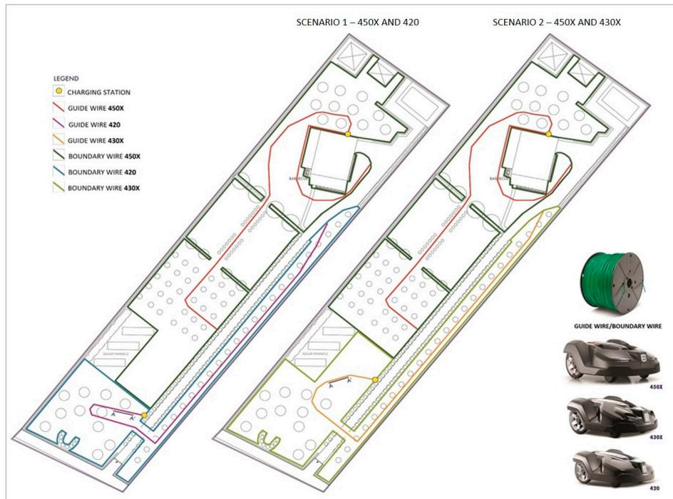
Figure 3. The two scenarios of management and the autonomous mowers involved in the study.
