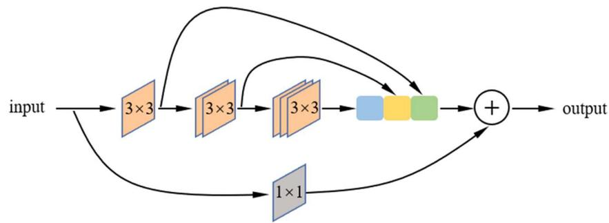
Figure 6. MultiResBlock structure.
