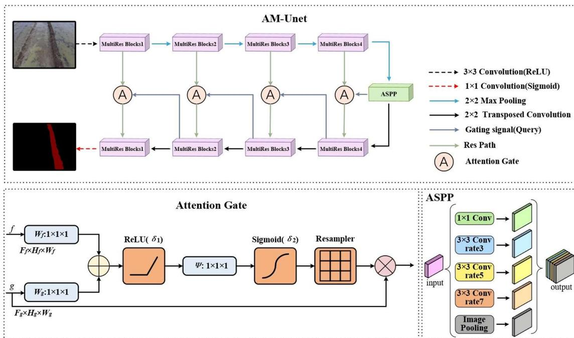
Figure 8. AM-UNet semantic segmentation model.
