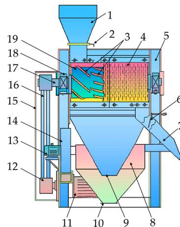
**Figure 4.** Oil-tea camellia seed sheller: (1) feed hopper; (2) feed regulating baffle plate; (3) spiral ribs and straight ribs; (4) cylindrical screen; (5) frame; (6) automatic dosing gate; (7) discharge port; (8) settling chamber; (9) fine shell outlet; (10) coarse shell outlet; (11) main motor; (12) belt pulley; (13) motor; (14) blower; (15) belt guard; (16) belt; (17) main shaft; (18) bearing block; (19) drum.
