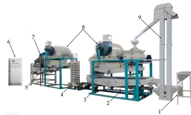
**Figure 16.** Flaxseed dehulling equipment TFYMZ-200: (1) input hopper; (2) main part of the equipment; (3) leaf-spring conveyor; (4) spiral elevator; (5) vibrating air-separator; (6) electric control cabinet; (7) electrostatic air separator; (8) vertical air-separating system; (9) bucket elevator.
