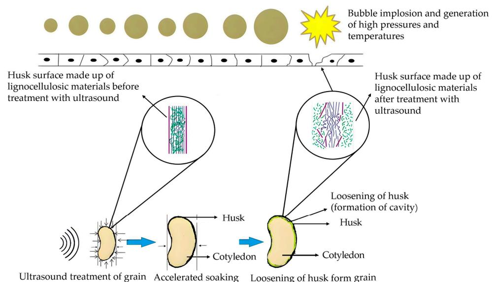
**Figure 12.** Ultrasonic dehulling principle.
