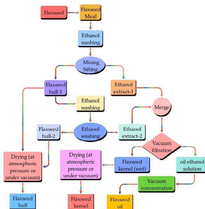
**Figure 2.** Ethanol dehulling process of flaxseed.
