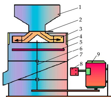
**Figure 6.** Rapeseed double impact husking test device: (1) hopper; (2) feed and adjustment set; (3) throwing plate; (4) dentiform circle; (5) secondary dehulling plate; (6) transmission shaft; (7) frame; (8) governor; (9) timing electrical machinery.
