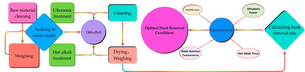
**Figure 13.** Ultrasonic-assisted lye peeling ultrasonic walnut kernel dehulling process flow.
