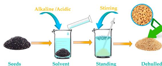
Figure 1. Chemical dehulling principle.
