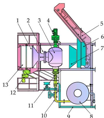
**Figure 11.** Structure diagram of steam sheller: (1) separator; (2) discharge port; (3) steam reaction tank; (4) motor; (5) mesh belt conveyor; (6) collection pond; (7) discharge port; (8) steam tank; (9) rack; (10) pipeline; (11) rotary joint; (12) gear motor; (13) driveshaft.
