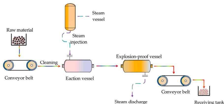
**Figure 10.** Steam explosion dehulling principle.
