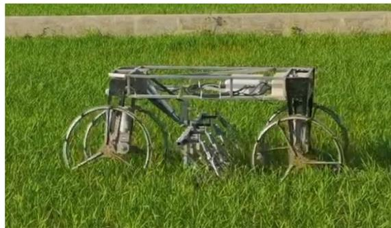
**Figure 12.** Field operation of mechanical weeder for organic rice.
