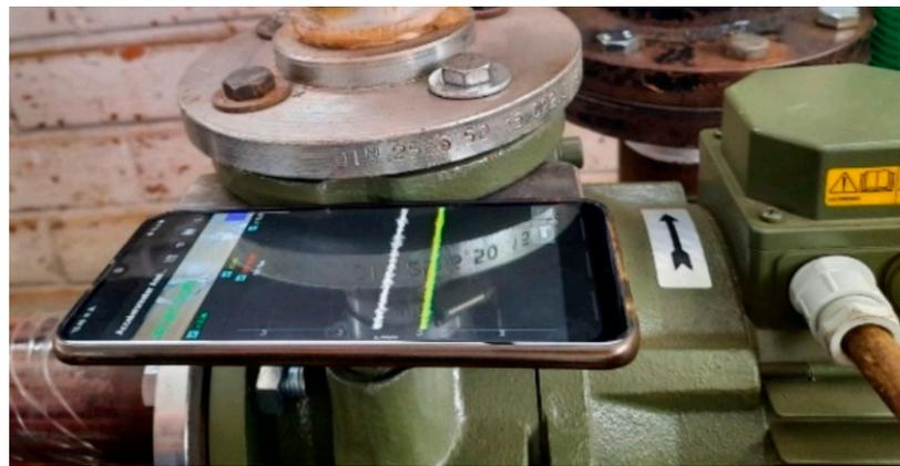
**Figure 3.** Actual mounting of the smart phone on the pump casing, using a rigid metal plate.
