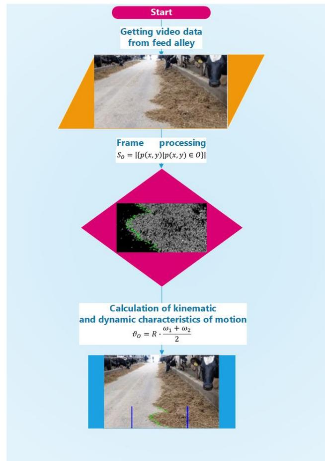
**Figure 2.** Functioning of the technical vision system for the robot feeder.
