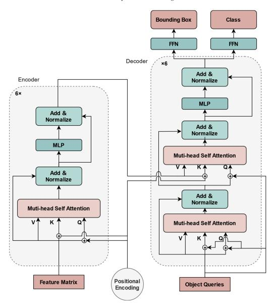
**Figure 6.** Transformer structure. The input features combined with the location encoding go through the Encoder and Decoder and finally output bounding box and class.
