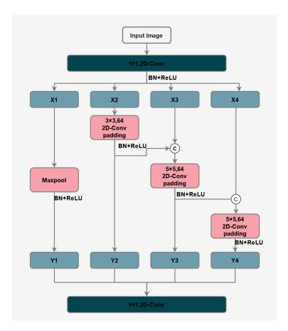
**Figure 4.** Res2Net Struct. Res2Net employs internal multi-scale convolution, which distinguishes it from ResNet.
