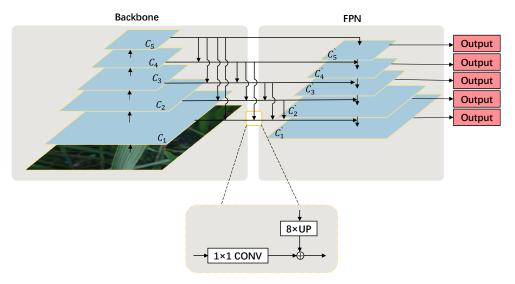
**Figure 5.** DHLC-FPN structure. DHLC-FPN employs Dense Higher-Level Composition multi-scale convolution, which distinguishes it from FPN.
