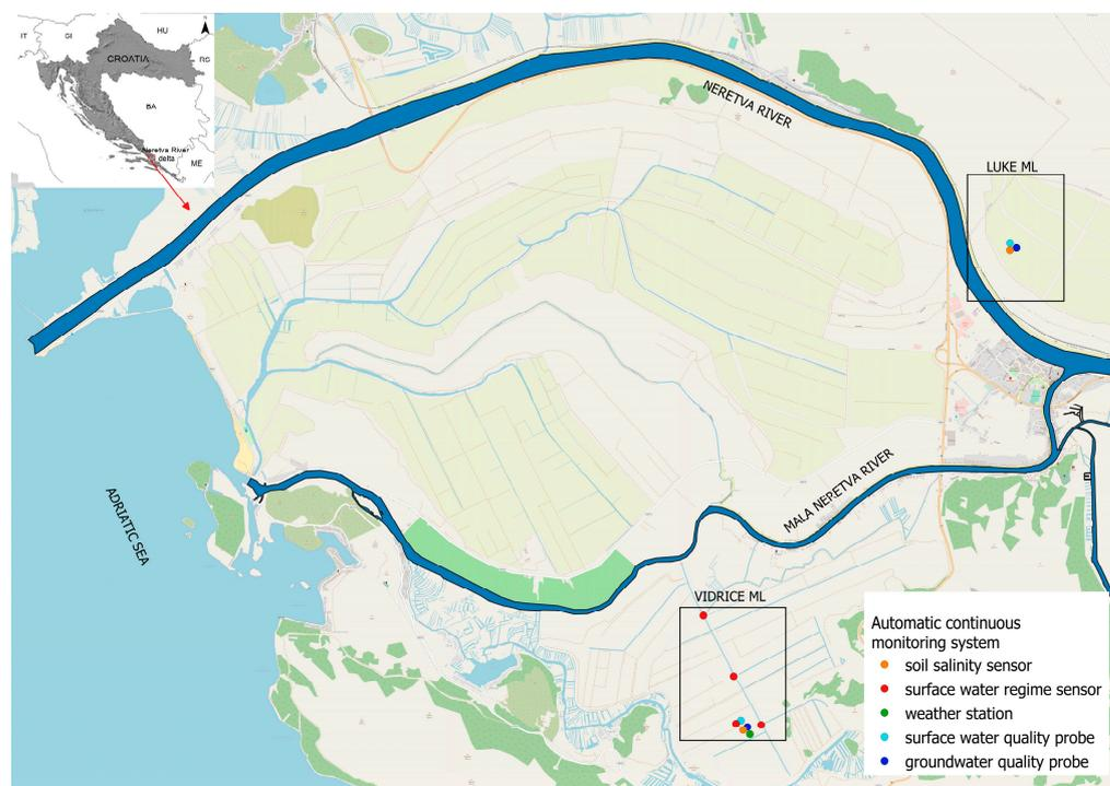
Figure 2. Project area and installed sensors (modified map form DELTASAL web portal).
