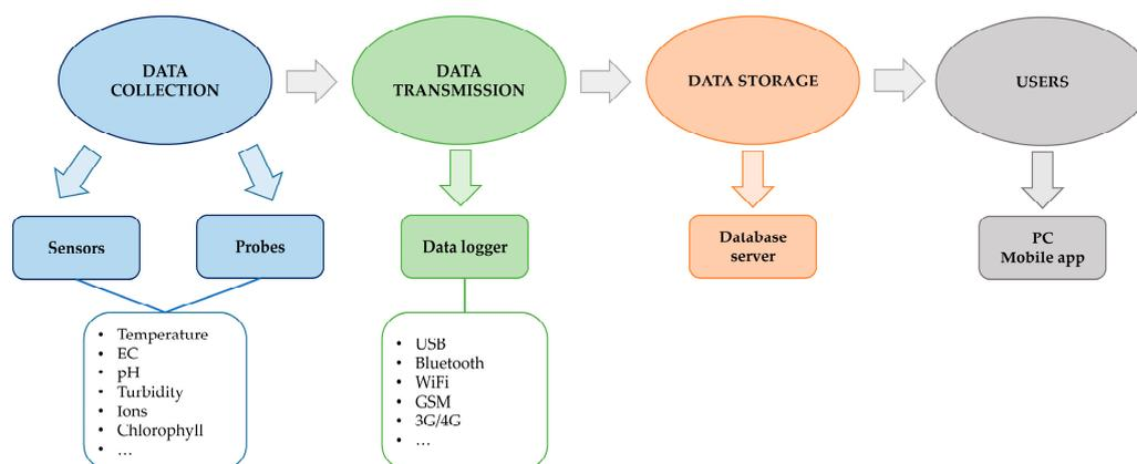
**Figure 1.** Scheme of automated continuous WQM.
