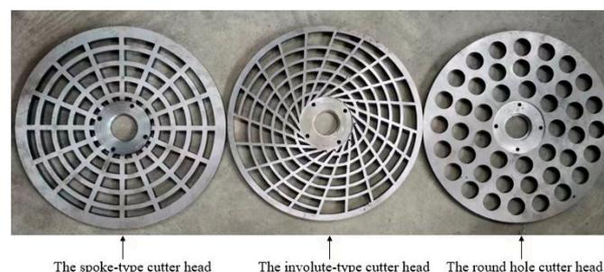
Figure 5. Three designed cutter heads.
