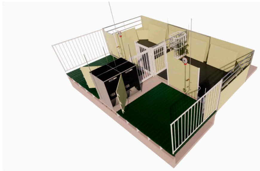
**Figure 9.** Slightly changed version of the SowComfort farrowing pen into a “from-farrowing- to-30 kg” pen where the litter can remain in their home pen until they are 30 kg. The pen has two feed dispensers and the entrance to the nest area is moved to one of the sides rather than in the middle to strengthen the walls and avoid an extra corner where piglets may choose to defecate and urinate. The drawing was constructed by May Helen Gryte in Fjøsssystemer A/S (2019).
