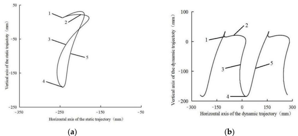
**Figure 6.** Trajectory of seedling picking after optimization: 1—The point of picking seedling; 2—The trajectory of clamping seedling stage; 3—The trajectory of holding seedling stage; 4—The point of planting seedling; 5—The trajectory of returning stage. (a) Static trajectory after optimization; (b) dynamic trajectory after optimization.
