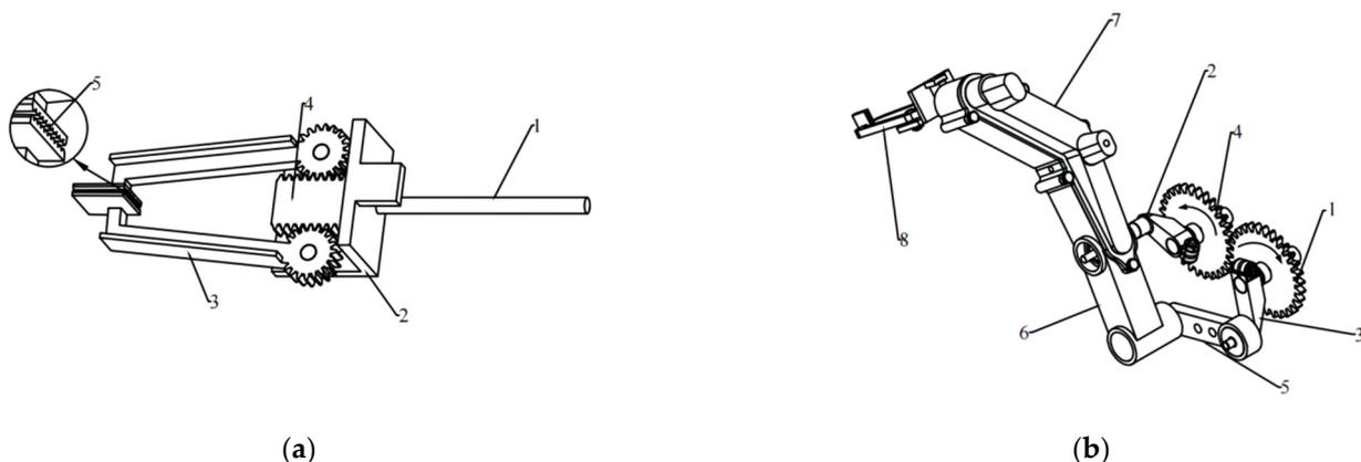
**Figure 2.** The automatic transplanting mechanism. (a) Flexible clamping mechanism. 1—Push rod; 2—rack mounting plate; 3—gripper; 4—rack; 5—wavy inner side. (b) Double-crank linkage mechanism. 1, 4—spur gear; 2, 3—crank; 5, 6, 7—connecting rod; 8—clamping mechanism.
