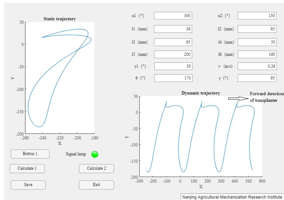
**Figure 4.** Parameter optimization program of clamping stem seedling picking mechanism.
