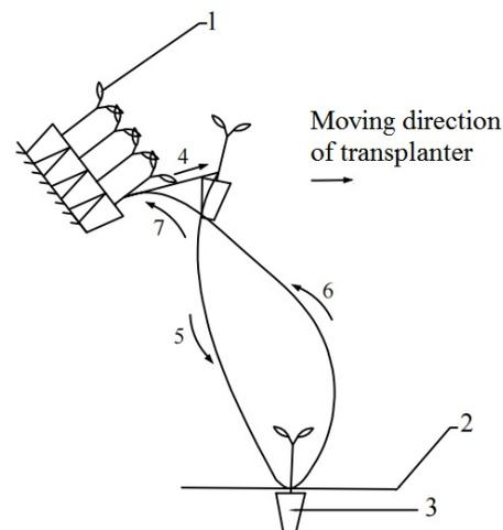
**Figure 1.** Backward transplanting movement trajectory planning: 1—hole tray seedling; 2—ground; 3—planting point; 4—picking seedling; 5—holding seedling; 6—returning; 7—clamping seedling.
