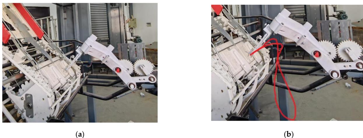
**Figure 7.** Actual trajectory of the seedling picking mechanism: (a) the prototype verification platform; (b) the actual seedling movement trajectory.
