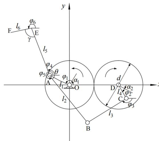
Figure 3. Motion diagram of double crank linkage mechanism.
