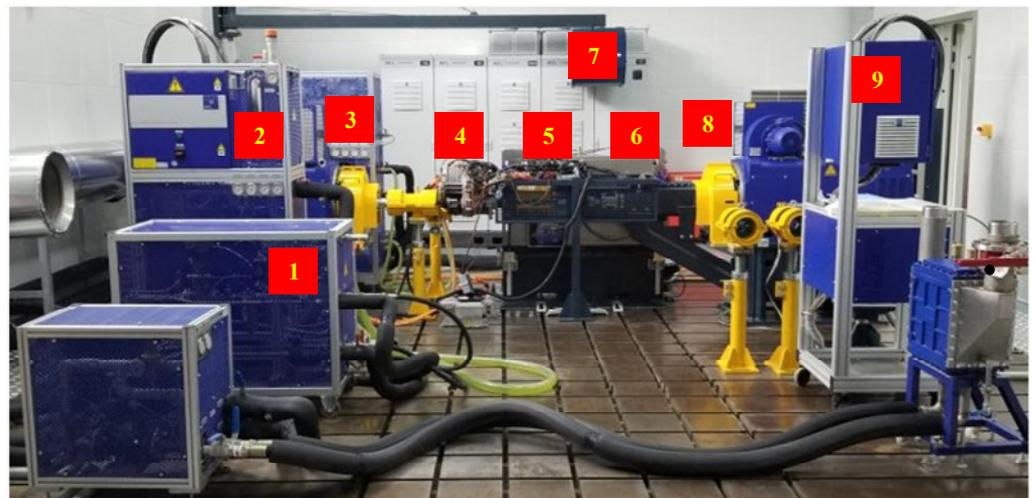
**Figure 14.** Test bench: 1. Oil cooling system; 2. motor cooling system; 3. variable frequency motor; 4. driving motor and coupling mechanism; 5. HMT; 6. central transmission device; 7. power cabinet of dynamometer; 8. electrical dynamometer; 9. data acquisition cabinet.
