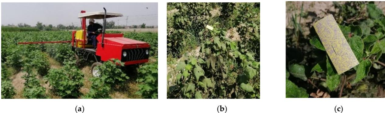
**Figure 2.** Field trials: (a) Sprayer in the cotton field during trials, (b) water-sensitive paper placement at the top of the plant canopy, (c) water-sensitive paper after spraying.
