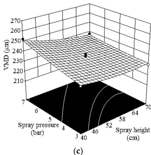
**Figure 12.** Three-dimensional surface map for VMD: (a) interaction effect of forward speed and spray height at 5 bar pressure; (b) interaction effect of forward speed and spray pressure at 55 cm height; (c) interaction effect of spray height and spray pressure at 6 km/h speed.
