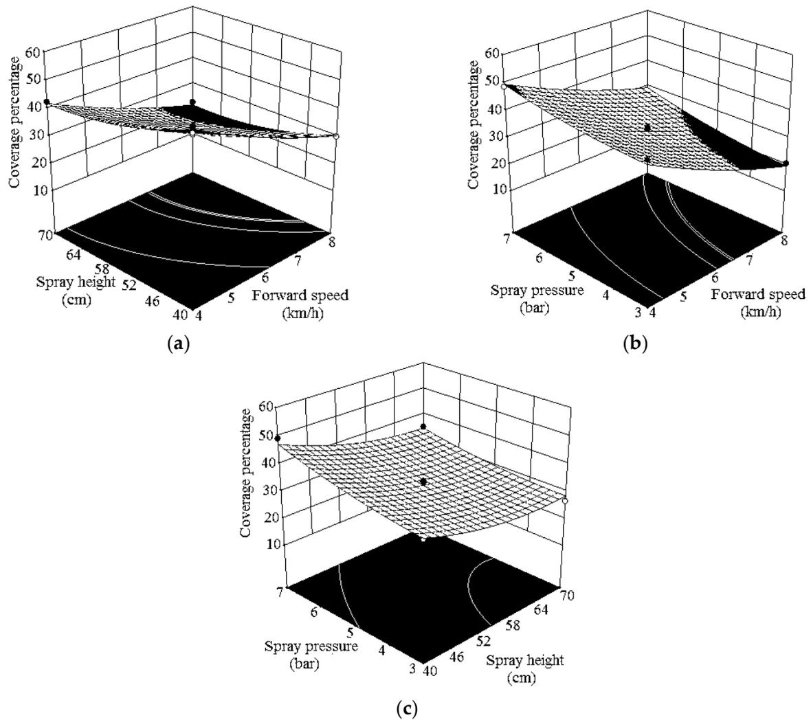
**Figure 11.** Three-dimensional surface map for coverage percentage: (a) interaction effect of forward speed and spray height at 5 bar pressure; (b) interaction effect of forward speed and spray pressure at 55 cm height; (c) interaction effect of spray height and spray pressure at 6 km/h speed.
