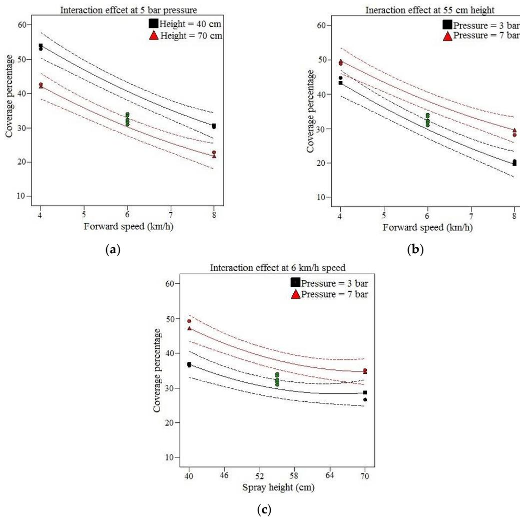
**Figure 8.** Coverage percentage: (a) relationship between forward speed and spray height at 5 bar pressure; (b) relationship between forward speed and pressure at 55 cm spray height; (c) relationship between spray height and pressure at 6 km/h speed.
