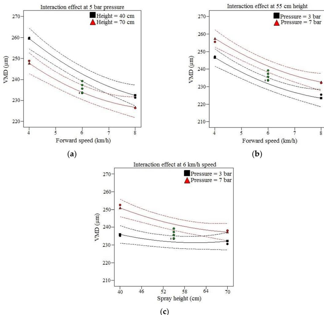
**Figure 9.** VMD: (a) Relationship between forward speed and spray height at 5 bar pressure; (b) Relationship between forward speed and pressure at 55 cm spray height; (c) relationship between spray height and pressure at 6 km/h speed.
