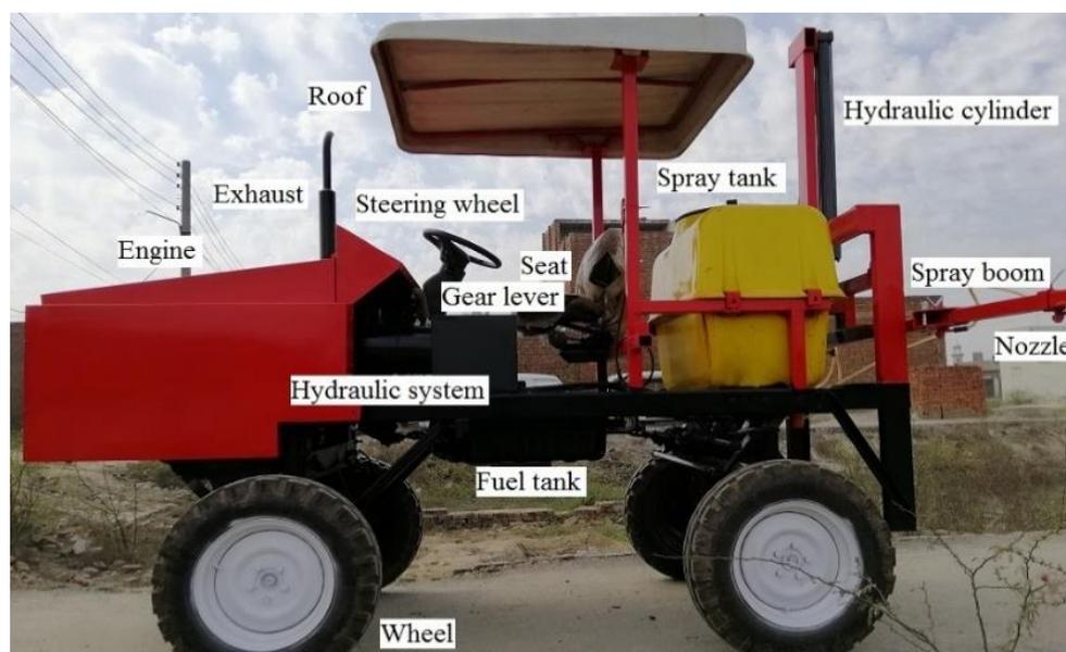
Figure 1. Self-propelled variable height crop sprayer.
