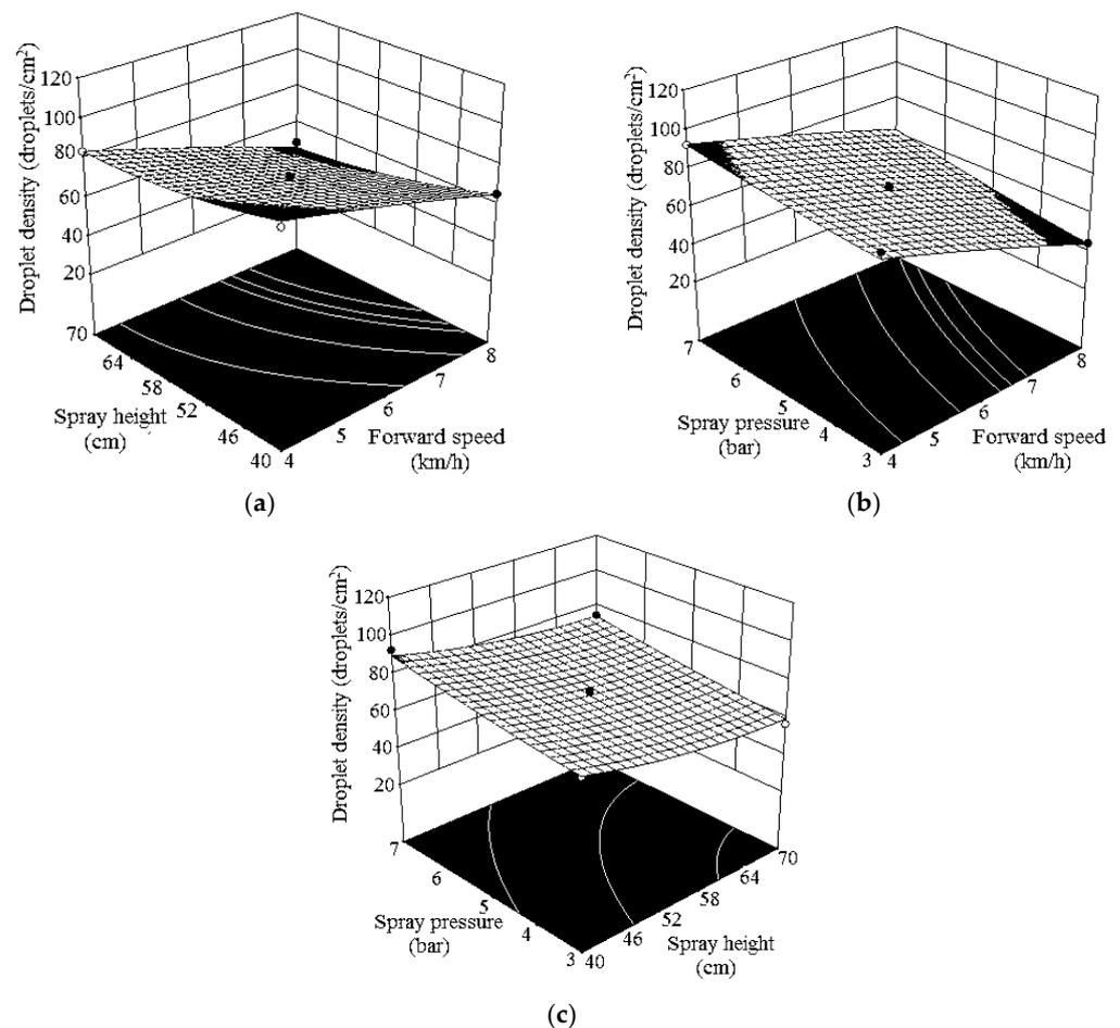
**Figure 10.** Three-dimensional surface map for droplet density: (a) interaction effect of forward speed and spray height at 5 bar pressure; (b) interaction effect of forward speed and spray pressure at 55 cm height; (c) interaction effect of spray height and spray pressure at 6 km/h speed.
