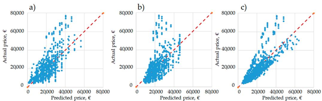
Figure 2. Qualitative evaluation for plough price prediction after application of linear models based on (a) working width, (b) power and (c) mass.
