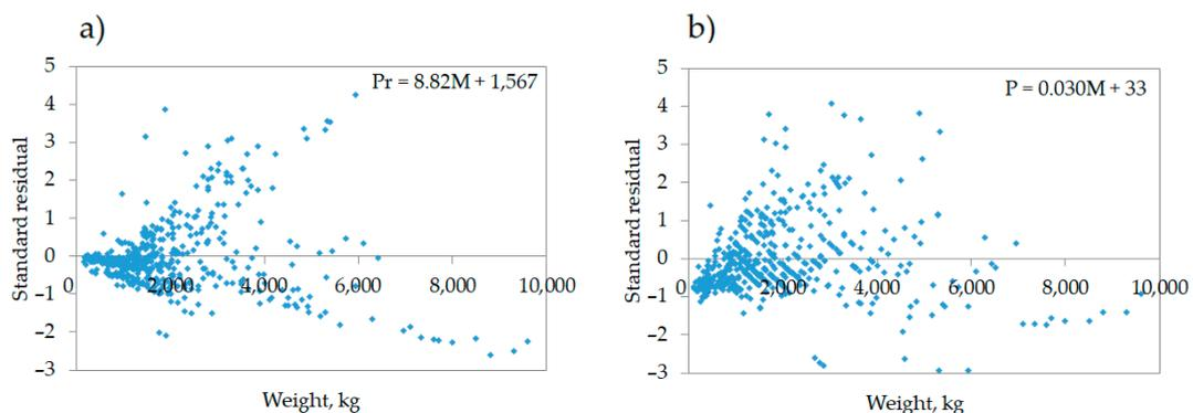
**Figure 3.** Plots of standard residuals based on the linear prediction models for price (a) and power (b) for harrows.
