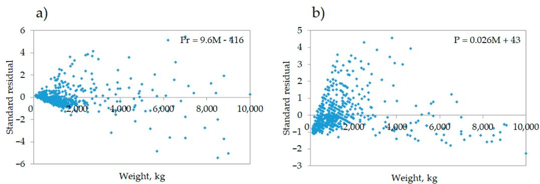
**Figure 5.** Plots of standard residuals based on the linear prediction models for price (a) and power (b) for cultivators.
