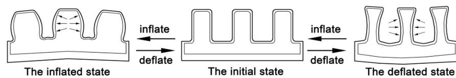
**Figure 4.** Schematic diagram of chamber deformation process.
