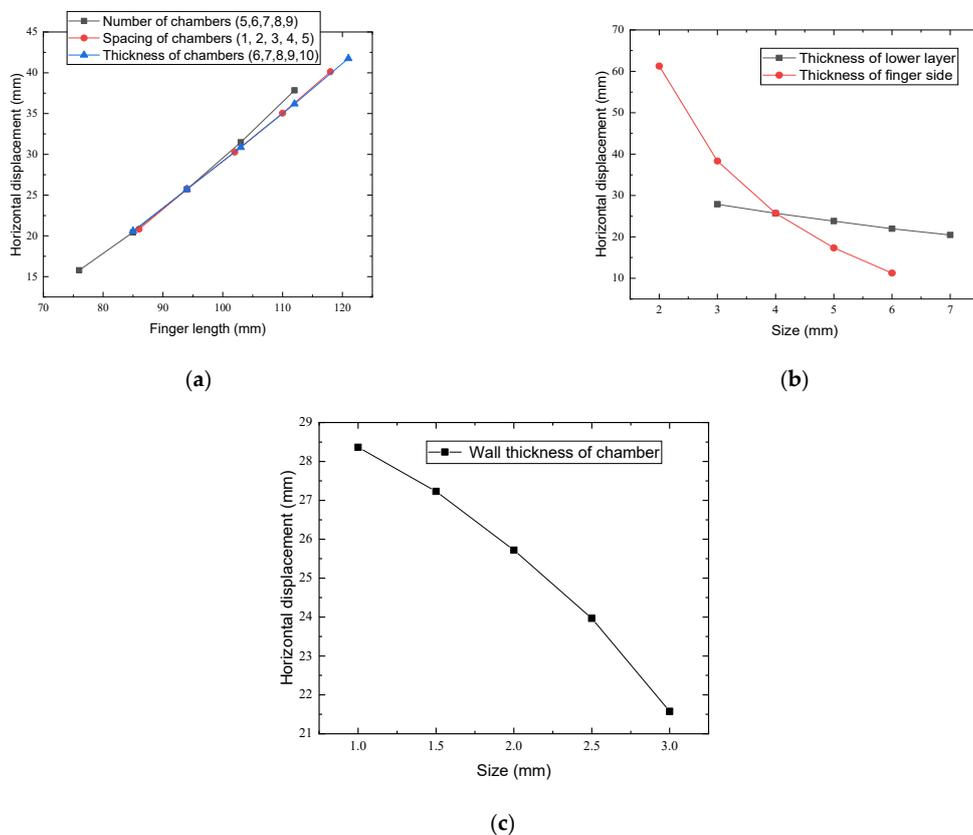
**Figure 12.** Simulation results: (a) shows the relationship between the spacing of chambers, the number of chambers, the thickness of chambers, and the horizontal displacement of finger ends; (b) shows the relationship between the thickness of finger bottom and the horizontal displacement of finger ends; (c) shows the relationship between the wall thickness of chambers and the horizontal displacement of finger ends.
