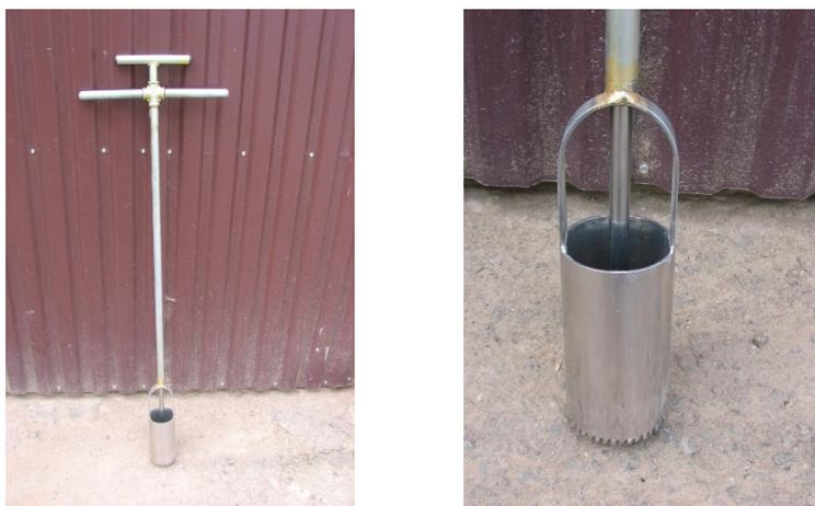
**Figure 1.** Soil sampling tube.
