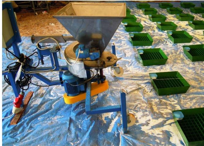
Figure 3. Disc spreader experimental test stand.
