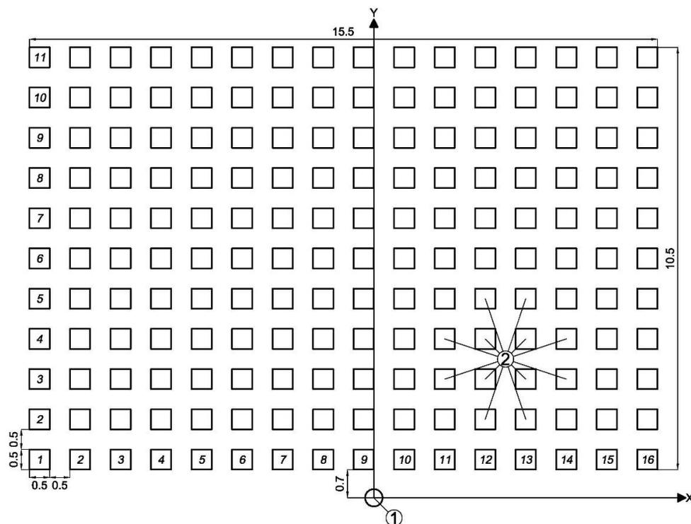
Figure 2. Scheme of experimental test site: (1) disc spreader; (2) collection trays.
