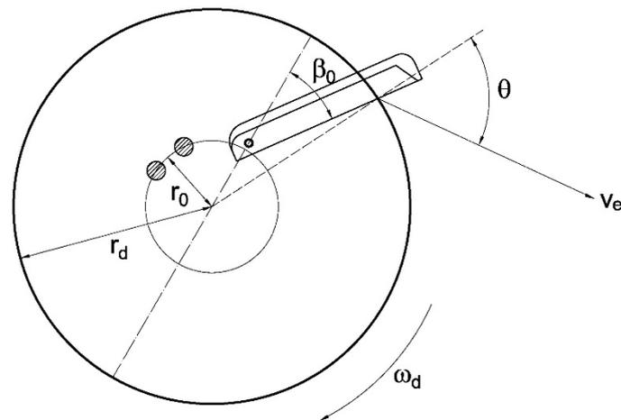
Figure 1. Geometry, kinematics, and dynamics of a spinning disc fertilizer.
