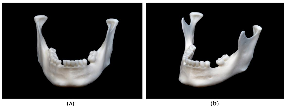
**Figure 4.** Mandibular model printed in stereolithography (SLA) technology: (a) front view; (b) side view.
