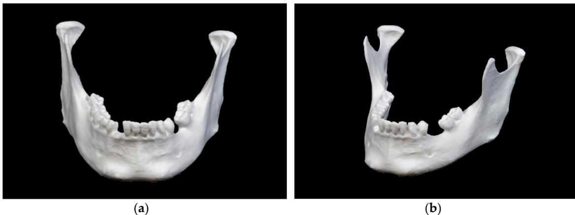
**Figure 3.** Mandibular model printed in fused filament fabrication (FFF) technology: (a) front view; (b) side view.
