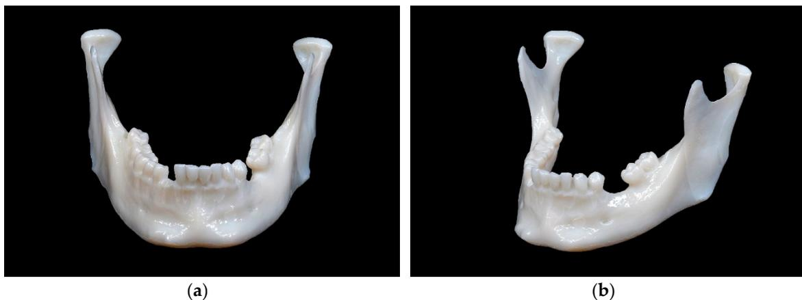
**Figure 6.** Mandibular model printed in material jetting (MJ) technology: (a) front view; (b) side view.
