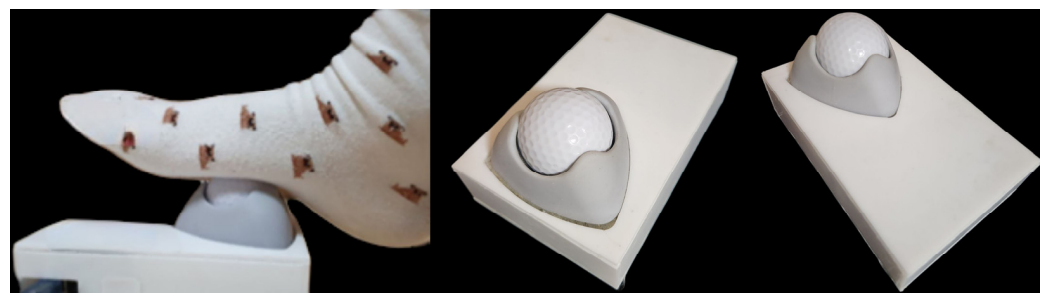
Figure 2. Application-linked massage ball sends information regarding the massage, such as the frequency and the force of massage on the foot, to the application in the patient's smartphone.
