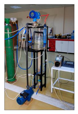
Figure 5. The developed membrane draft tube jet loop reactor.
