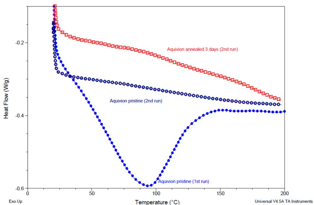
**Figure 7.** Differential scanning calorimetry (DSC) curves of Aquivion<sup>®</sup> 870 before (blue) and after annealing at  $140\text{ }^{\circ}\text{C}$  in presence of DMSO for 3 days (red).
