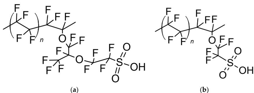
**Figure 1.** (a) Long side chain perfluorosulfonic acid (LSC-PFSA) Nafion<sup>®</sup> 1100 ( $n = 6.6$ ) and (b) short side chain PFSA (SSC-PFSA) Aquivion<sup>®</sup> 830 ( $n = 5.5$ ).
