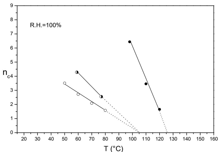
**Figure 5.**  $n_c/T$  plot of un-crystallized Aquivion<sup>®</sup> 830: as cast (empty circles), after treatment at 135 °C for 15 h (half empty circles) and treated at 135 °C for 15 h and annealed at 135 °C in presence of DMSO for 7 days (full circles).
