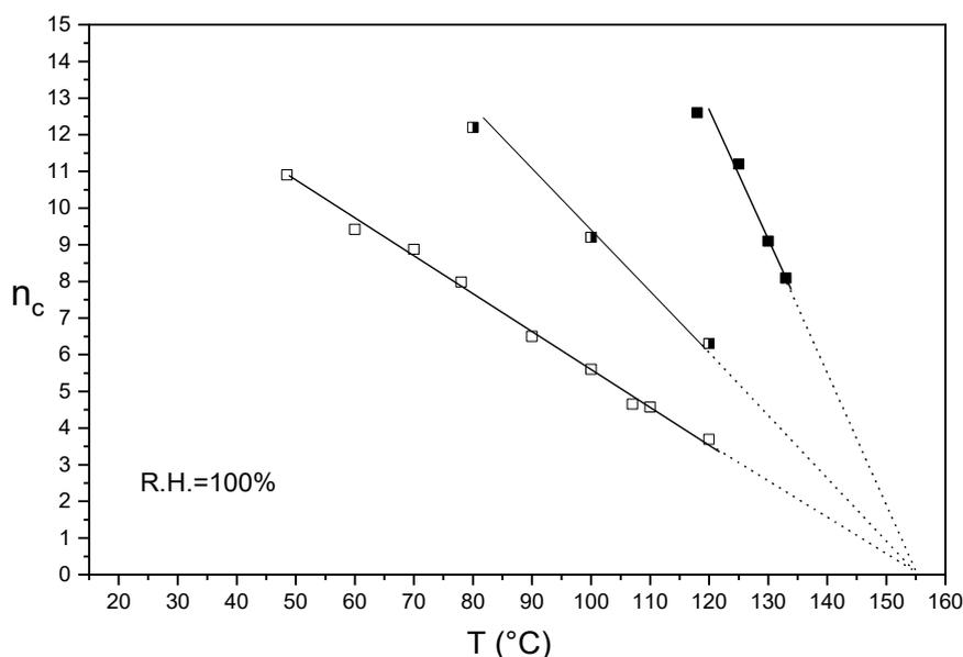
**Figure 2.**  $n_c/T$  plot of semi-crystalline Aquivion® 870 before (empty squares) and after annealing at 140 °C in presence of DMSO for 3 (half empty squares) and 7 days (full squares).
