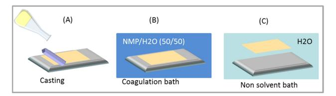
**Figure S2.** Schematic of the phase inversion steps: (A) polymer solution casting on clean glass plate; (B) System immersed in a coagulation bath with solvent mixture 50:50% of NMP: water; (C) Glass plate with the formed PBI support immersed into pure water.
