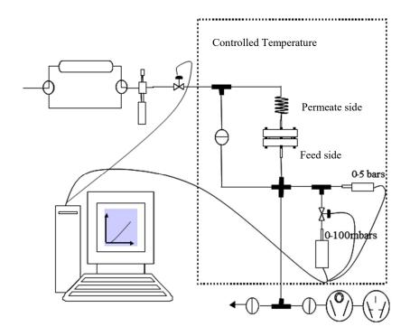
Figure S3. Schematic of the lab-scale experimental set-up used for single gas permeation measurements.
