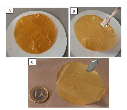
**Figure S1.** Photos of the prepared SILMs: A) IL based SILM (RPBI-IL); B) MIL based SILM (RPBI-MIL); C) PIL based SILM (RPBI-PIL).
