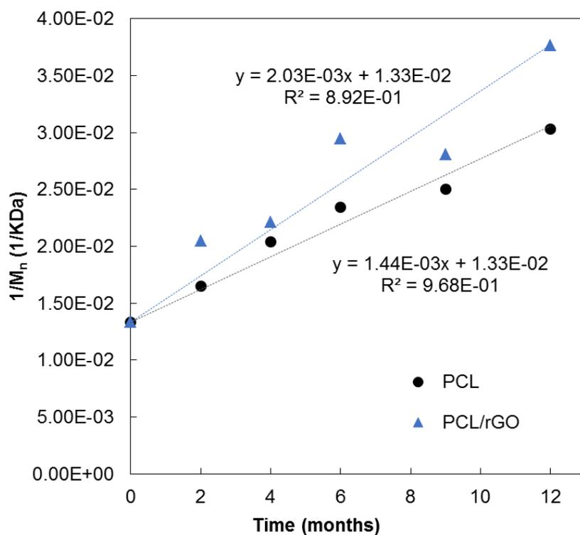
**Figure S1.** Kinetics of the hydrolysis of PCL and PCL/rGO membranes. Fitting of the molecular weight to the 2nd order hydrolysis kinetics (Equation S2) is depicted (dotted lines). For the present system  $M_0$  and  $C_w$  are the same for the PCL plain membranes and the PCL/rGO material as well as  $M_n0$ . Therefore from Figure S1, it can be extracted that  $k(\text{PCL})/k(\text{PCL/rGO}) = (2.03 \times 10^{-3})/(1.44 \times 10^{-3}) \approx 1.4$ .
