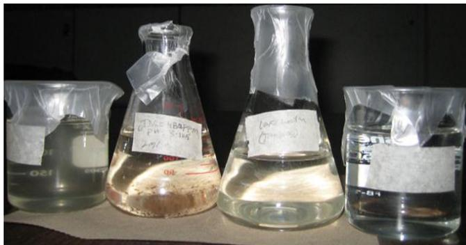
**Table 4.** Turbidity, pH, and TDS values of lake water as function of Alum addition after 1 h and 24 h settlements by gravity.
