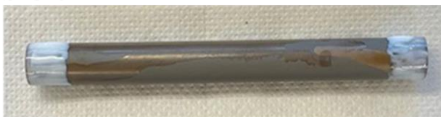
Figure S1. SiC membranes after ageing in NaClO for 200hrs.
