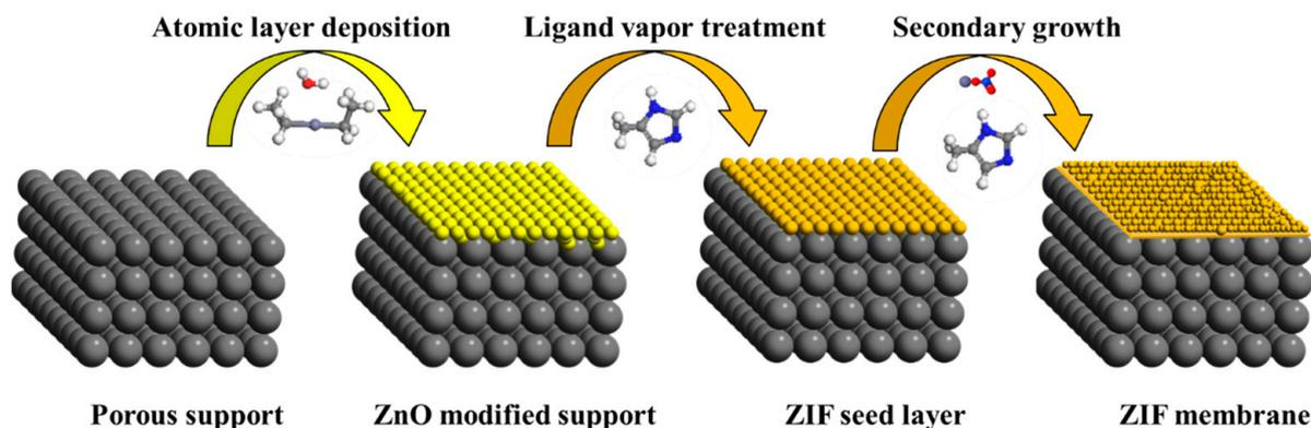
**Figure 1.** A schematic illustration depicting the procedures for fabricating ZIF membranes using vapor-phase seeding and secondary growth.
