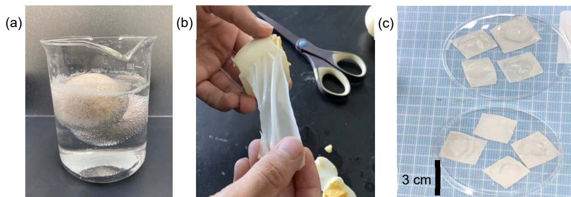
Figure S1. Preparation of the ESM. (a) the boiled egg immersed in 2 M HCl. (b) The belt-like ESM. (c) The square-shaped ESM.
