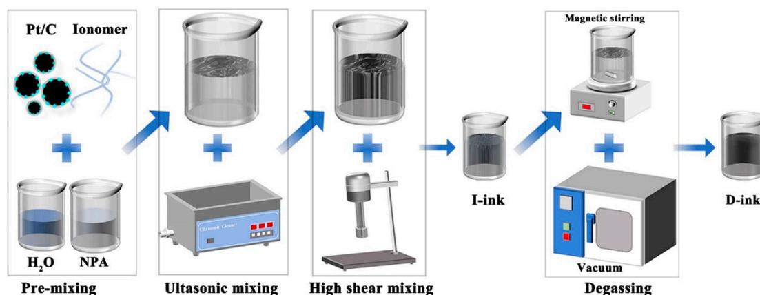
**Figure 1.** Schematic representation of the process of HSC ink preparation.
