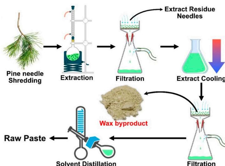
Figure 1. Schematic representation of pine needle extraction process.
