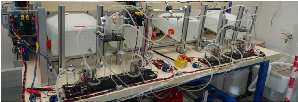
Figure 1. Test bench with four H-Tec PEM “Electrolyzer H<sub>2</sub>/O<sub>2</sub> 65”.
