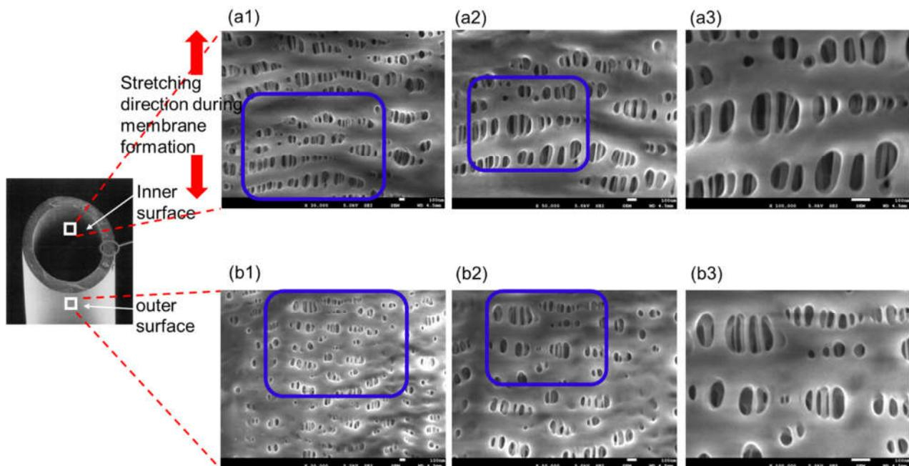
**Figure 3.** FE-SEM images of oxia<sup>®</sup> (dry), (a) the surface of inner lumen of the capillary membranes, (b) the outer surface of the capillary membranes: (1)  $\times 30,000$ ; (2)  $\times 50,000$ ; and (3)  $\times 100,000$ , respectively. The image of (3) shows magnified images of the pores enclosed by the blue square in (2), and the image of (2) shows magnified images of the pores enclosed by the blue square in (1).
