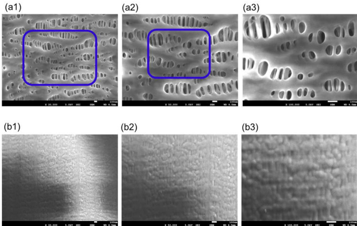
**Figure 4.** FE-SEM images of MERA NHP<sup>®</sup> (dry), (a) the surface of inner lumen of the capillary membranes, (b) the outer surface of the capillary membranes: (1)  $\times 30,000$ ; (2)  $\times 50,000$ ; and (3)  $\times 100,000$ , respectively. The image of (3) shows magnified images of the pores enclosed by the blue square in (2), and the image of (2) shows magnified images of the pores enclosed by the blue square in (1).
