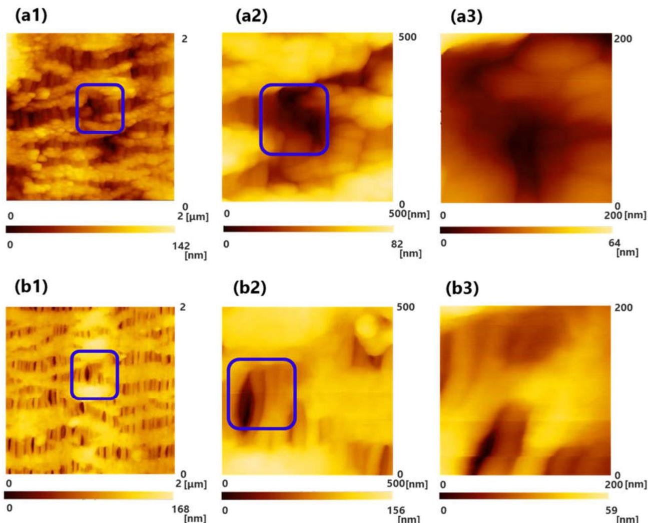
**Figure 2.** Scanning probe microscopy (SPM) images of oxia<sup>®</sup> (dry), (a) the surface of inner lumen of the capillary membrane, and (b) the outer surface of the capillary membrane: (1) 2000 nm × 2000 nm; (2) 500 nm × 500 nm; and (3) 200 nm × 200 nm, respectively. The image of (3) shows magnified images of the pores enclosed by the blue square in (2), and the image of (2) shows magnified images of the pores enclosed by the blue square in (1).
