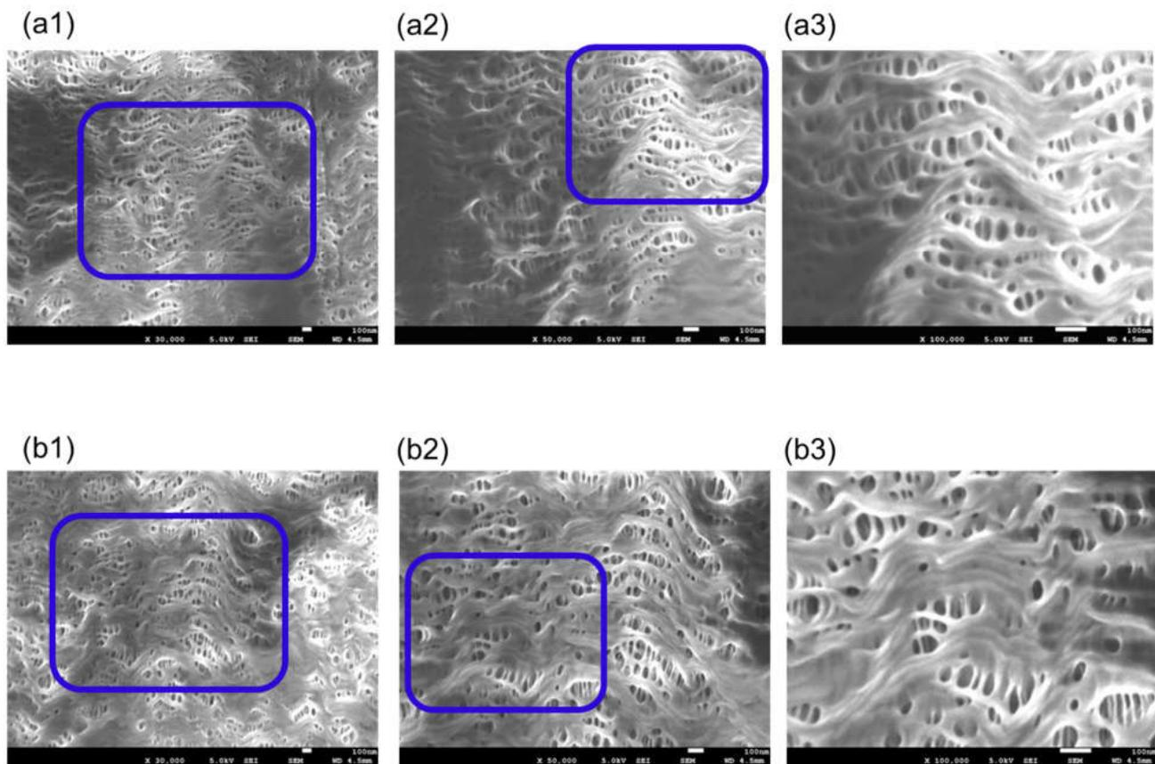
**Figure 7.** FE-SEM images of BIOUCUBE<sup>®</sup> (dry), (a) the surface of inner lumen of the capillary membranes and (b) the outer surface of the capillary membranes: (1)  $\times 30,000$ ; (2)  $\times 50,000$ ; and (3)  $\times 100,000$ , respectively. The image of (3) shows magnified images of the pores enclosed by the blue square in (2), and the image of (2) shows magnified images of the pores enclosed by the blue square in (1).
