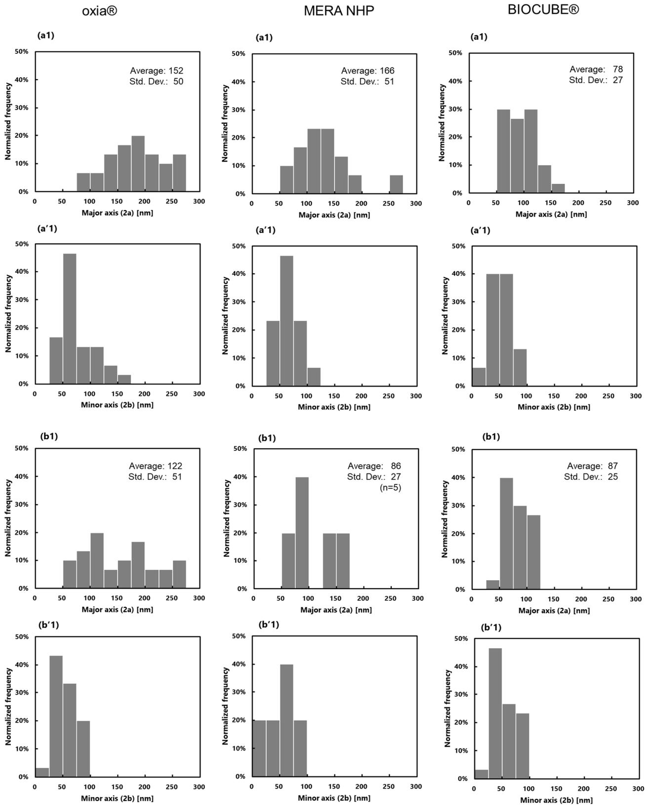
**Figure 8.** Distribution of the ellipse pore diameter of three membranes (dry), determined via FE-SEM, (a) the surface of inner lumen of the capillary membranes and (b) the outer surface of the capillary membranes. (a1,b1) Major axis (2a), (a'1,b'1) Minor axis (2b).
