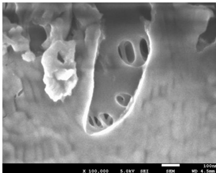
**Figure 5.** FE-SEM image of MERA NHP<sup>®</sup> (dry), the outer surface of the capillary membranes; and  $\times 100,000$ .
