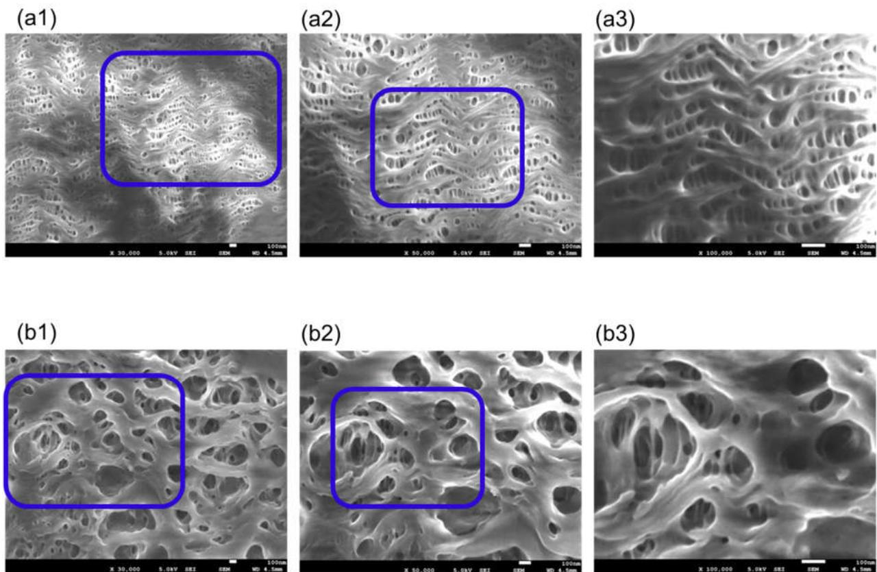
**Figure 6.** FE-SEM images of BIO-CUBE<sup>®</sup> (dry), (a) the surface of inner lumen of the capillary membranes and (b) the outer surface of the capillary membranes: (1)  $\times 30,000$ ; (2)  $\times 50,000$ ; and (3)  $\times 100,000$ , respectively. The image of (3) shows magnified images of the pores enclosed by the blue square in (2), and the image of (2) shows magnified images of the pores enclosed by the blue square in (1).
