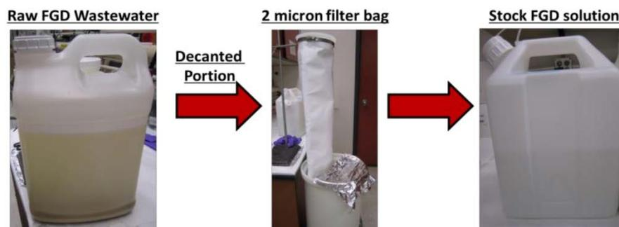
**Figure 4.** Preparation of stock FGD WW solution. Raw FGD WW was allowed to settle and then decanted. The decanted portion was filtered through a filter bag to produce the stock FGD solution. This stock solution was diluted for RO studies.
