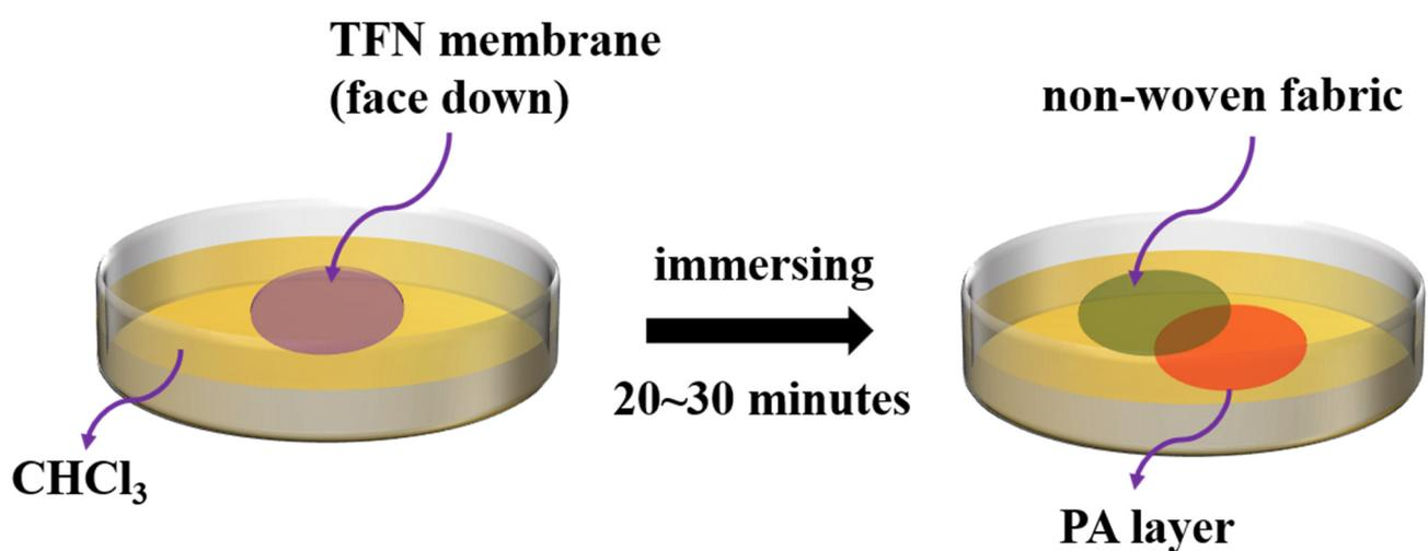
**Figure S2.** PA layer back transfer process.
