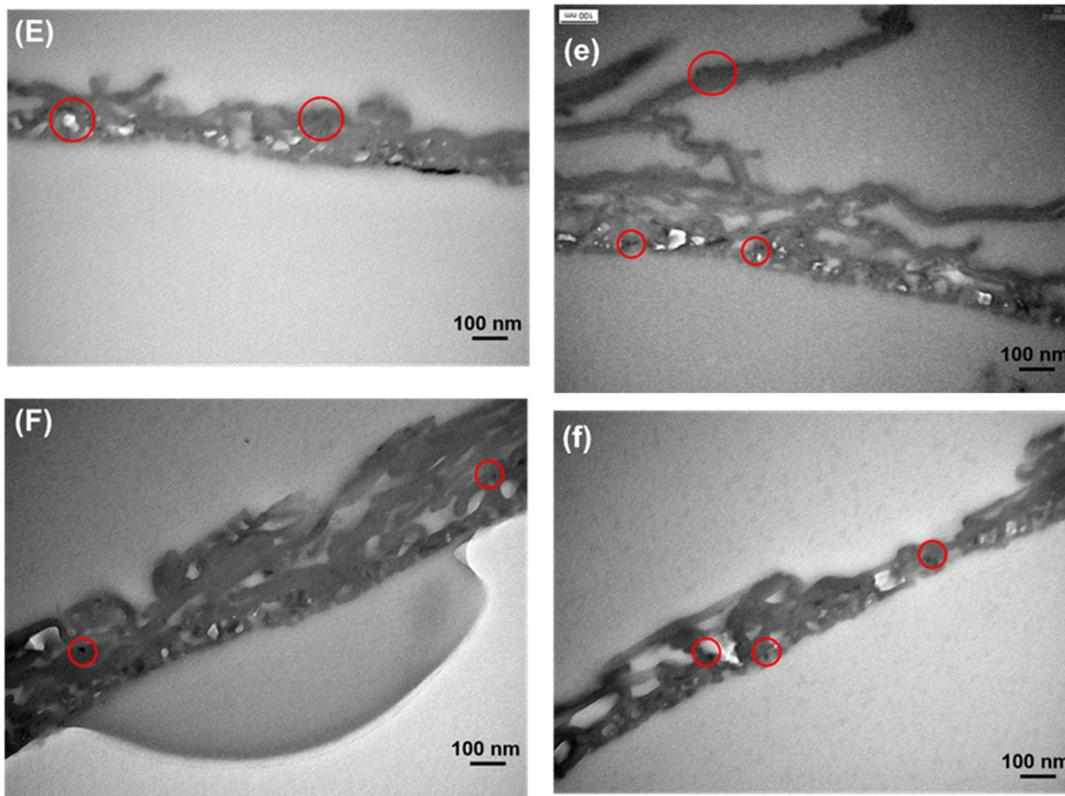
**Figure S1.** TEM images of the membranes with different PTS loading: (A, a) TFC membrane; (B, b) TFN-0.1 membrane; (C, c) TFN-0.2 membrane; (D, d) TFN-0.3 membrane; (E, e) TFN-0.4 membrane; (F, f) TFN-0.5 membrane.
