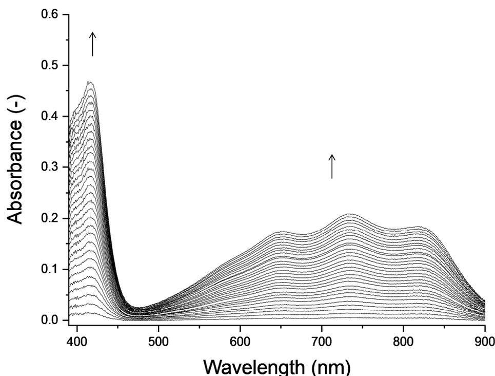
**Figure S4.** Changes of the absorption spectrum of the reaction solution as a function of reaction time, with  $[ABTS^{2-}]_0 = 0.25$  mM,  $[H_2O_2]_0 = 80$   $\mu$ M and  $[HRP] = 150$  pM at 25 °C (10 mM MES buffer pH = 5). The spectra were recorded at intervals of 10 sec immediately after the start of the reaction (up to 5 min).
