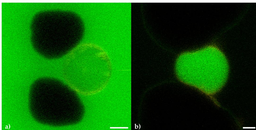
**Figure S2.** (a) Wide-field fluorescence image of a single GUV trapped hydrodynamically by the posts (black). Scale bar 5000 nm. The surrounding calcein solution (green) is diverted around the trap (b). The fluid was then exchanged for water without removing the calcein filled GUV. Scale bar 2000 nm.
