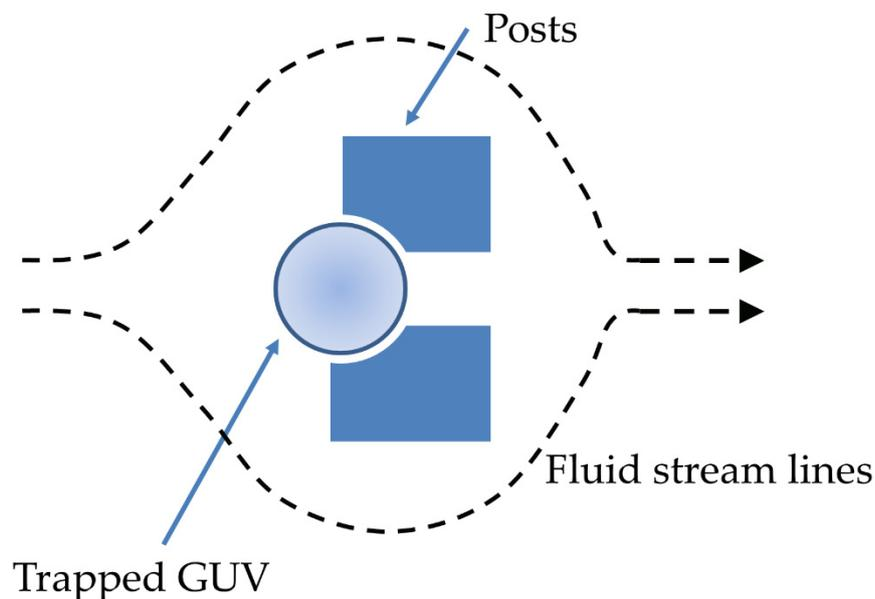
**Figure S1.** Scheme showing a trapped GUV isolated and the fluid flow around the trap. The chip and the valves are not shown in the figure, for details see ref [1].
