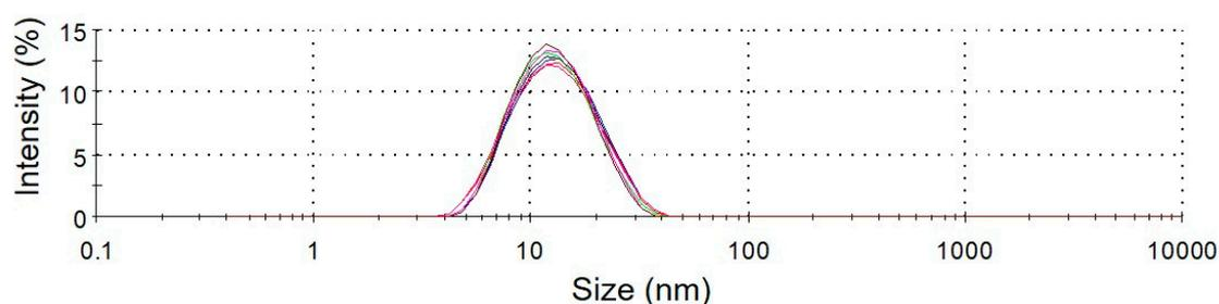
**Figure S1.** Size distribution of DLPC/deoxycholic acid micelles measured in 1.0 mM HEPES buffer (pH 7.4) using a Zetasizer Nano ZS ZS90 (Malvern Instruments Ltd, Worcestershire, UK).
